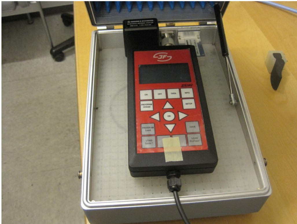
Photo 4.4.1 Test setup regarding measurement of 20 dB bandwidth.
