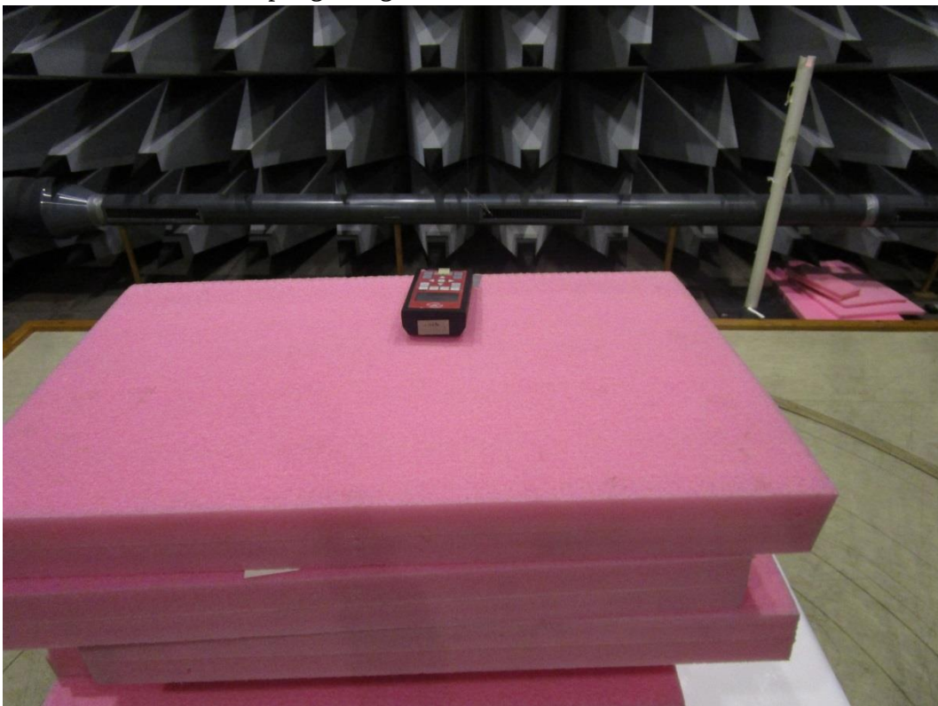
Photo 4.1.2 Test setup regarding measurement of radiated emission.
