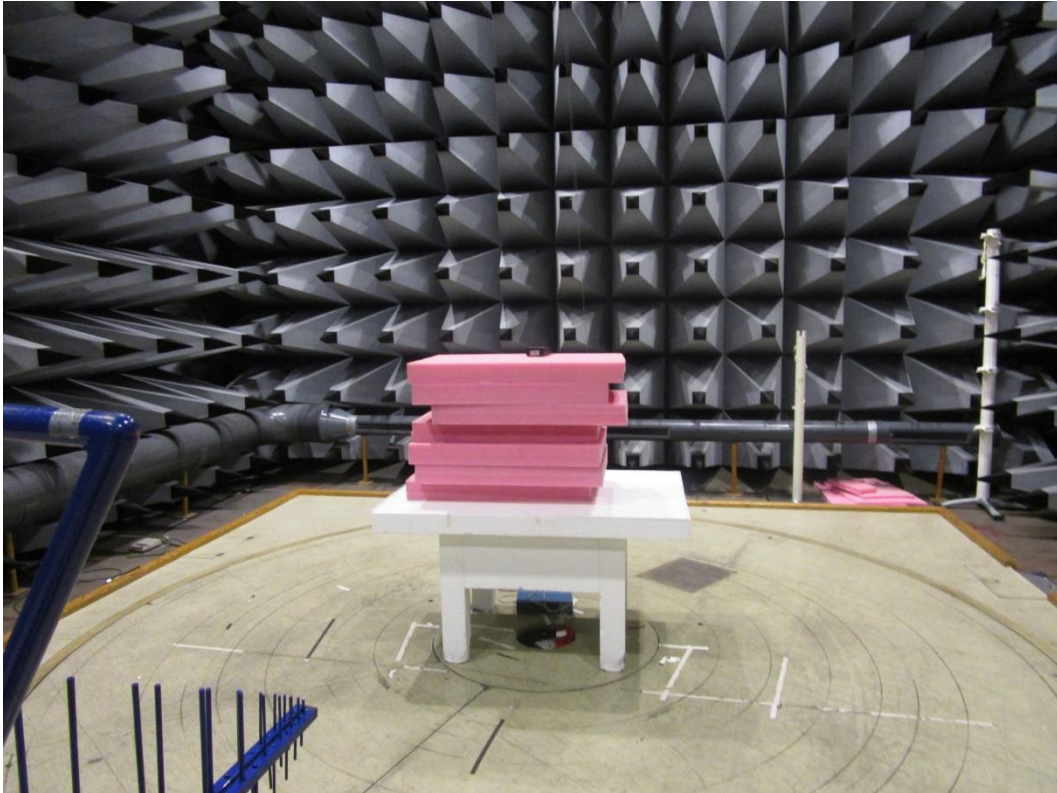
Photo 4.3.1 Test setup regarding measurement of band edge compliance.
