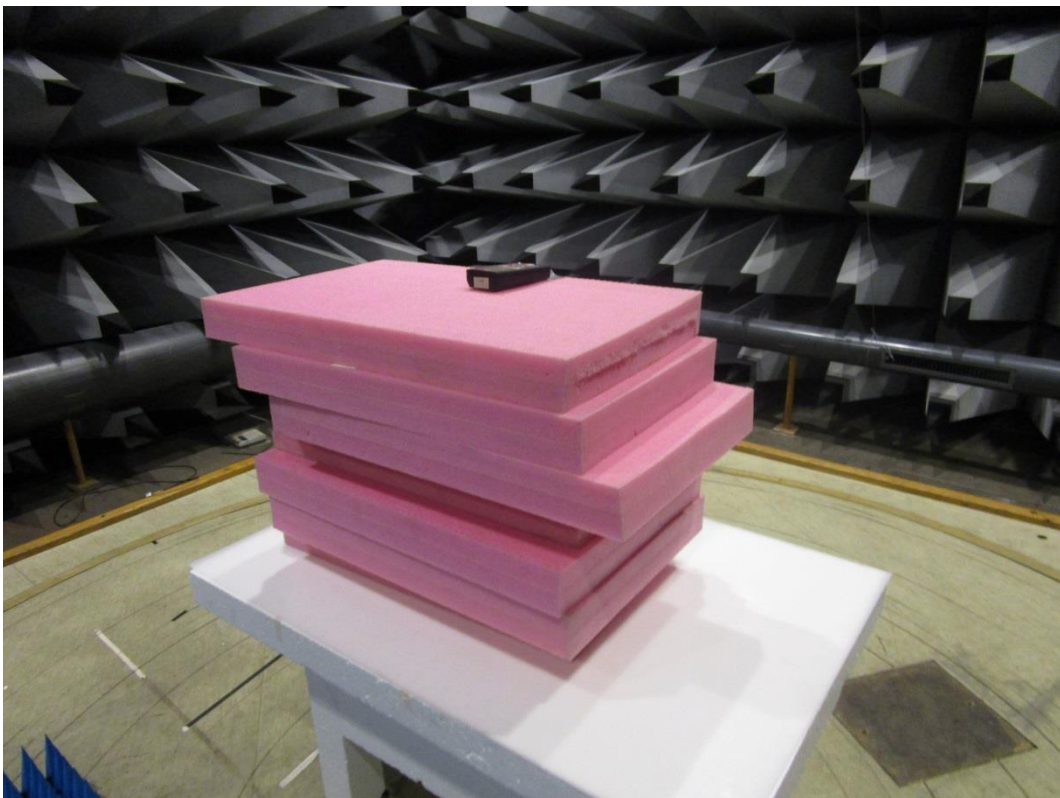
Photo 4.1.4 Test setup regarding measurement of radiated emission.
