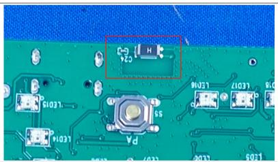
The antenna is Chip antenna.
