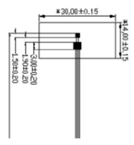
Figure 1 Physical dimension (mm)
