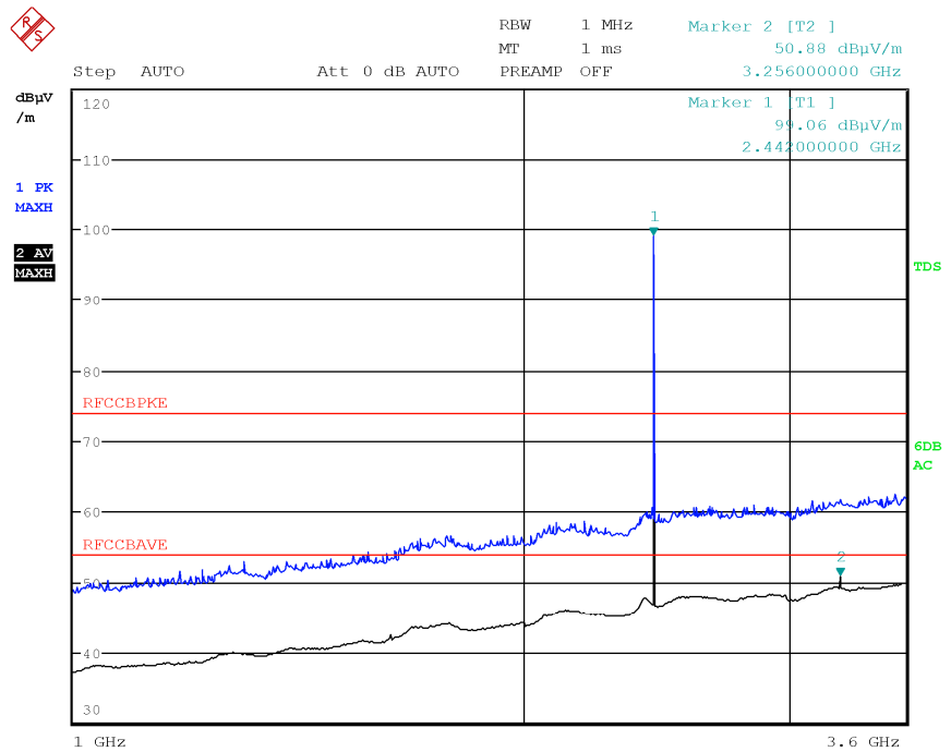
Figure 8.5-16: Radiated spurious emissions 1 to 3.6 GHz, Mid channel BLE with antenna in vertical polarization
