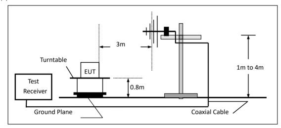
(c) For radiated emissions above 1000MHz
