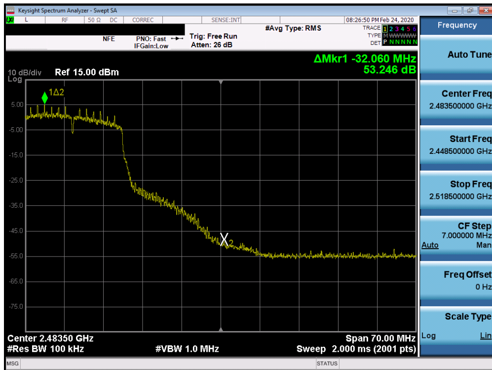
Plot 7-27. Band Edge Plot (802.11n (2.4GHz) – Ch. 10)
