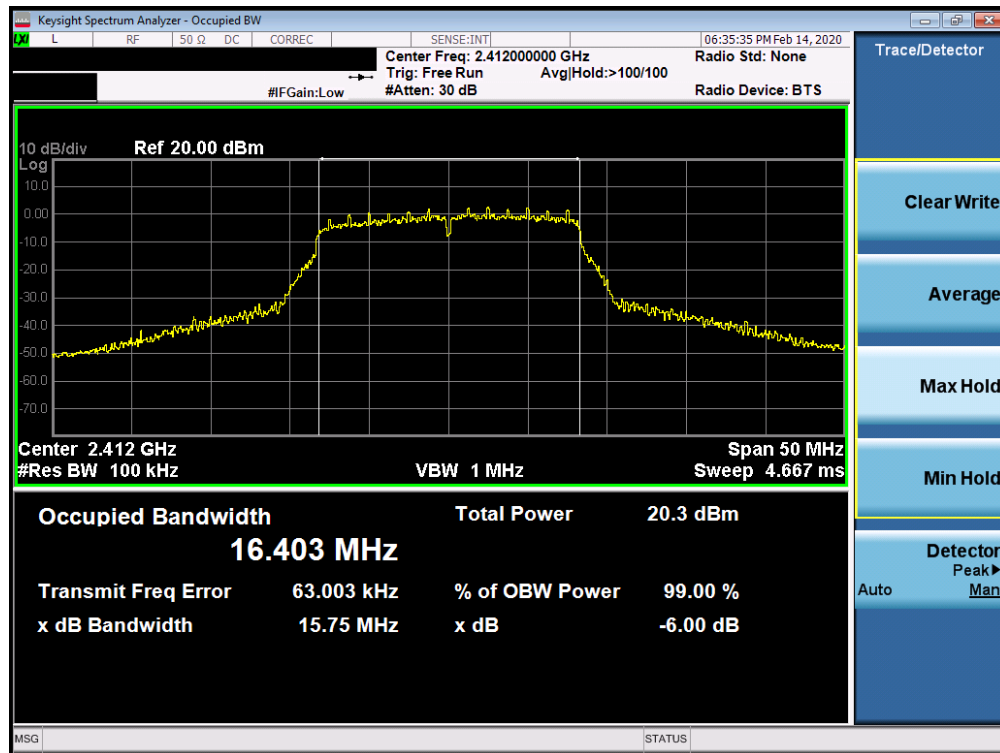
Plot 7-4. 6dB Bandwidth Plot (802.11g – Ch. 1)
