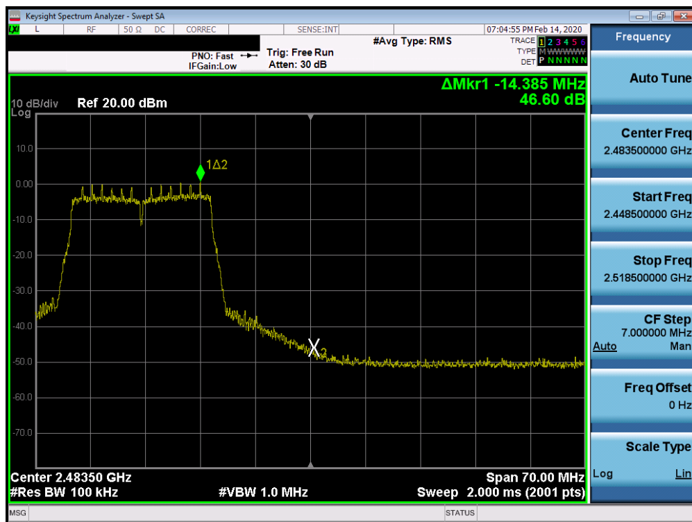
Plot 7-28. Band Edge Plot (802.11n (2.4GHz) – Ch. 11)
