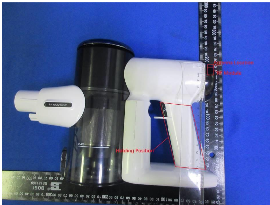
View of RF Module& Antenna location
