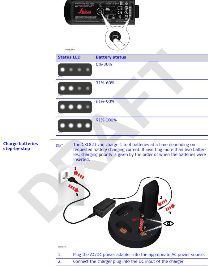
3. Insert the battery with the contact slots facing downwards.
