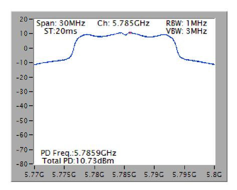
Power Density Plot on Configuration IEEE 802.11n MCS0 HT20 / Chain 1 + Chain 2 / 5785 MHz
