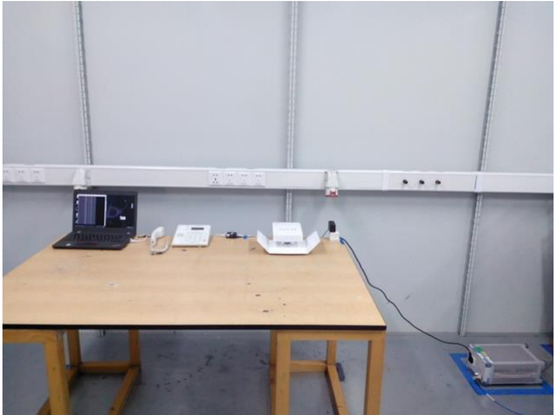
AC Conducted Emission Test Setup -Front
