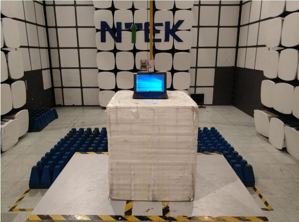
**Radiated Measurement Photos ( new battery )**
