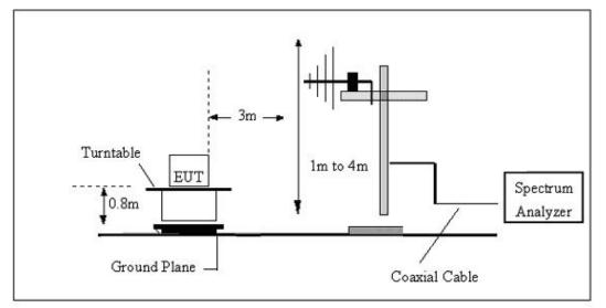
(C) Radiated Emission Test-Up Frequency Above 1GHz
