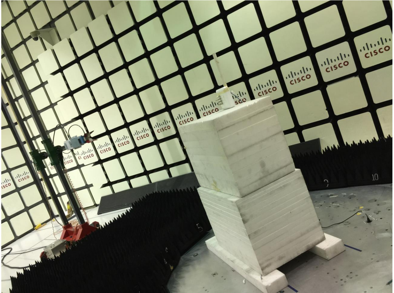
AIR-AP3802I-B-K9 Radiated Emissions setup above 1GHz
