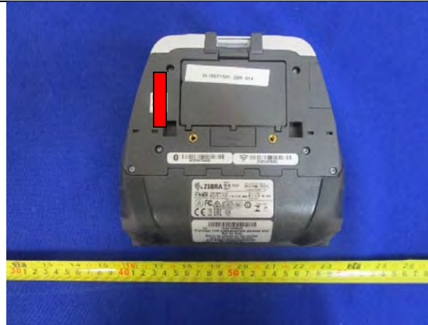
Test Position-1 (Bottom Side with 0mm distance)
