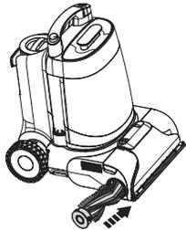
Place the brush roller back by inserting the brush roller end into the right side of the holder, then attach the roller tab to the left side to lock into place.
