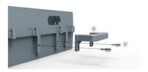
2. Attach and fasten the Bracket I to the left side of M2RU with screws M6×14 using T5 Wrench.
