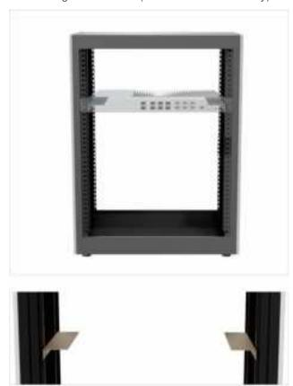
3. Place the EU in the rack and secure the EU using 2 screws M6×16 on both sides and the Phillips screwdriver.
