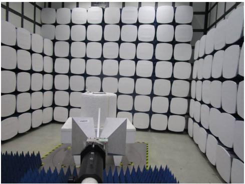
1.3 Radiated Spurious Emissions Test Setup
