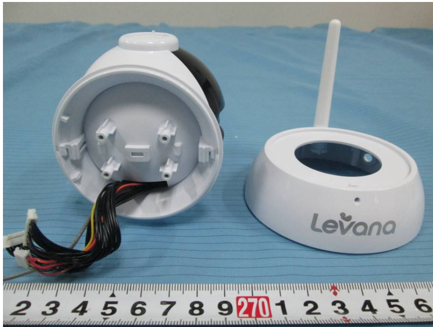
EUT – Cover off View 3
