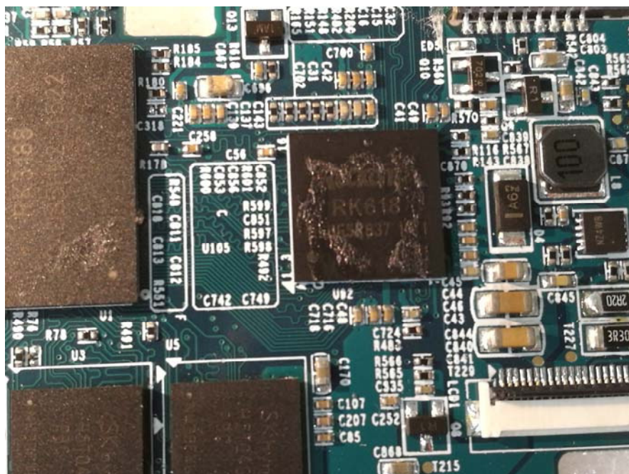
EUT – Main IC View 3
