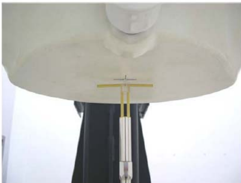
Fig 7.2 Setup Photo of Dipole Antenna
