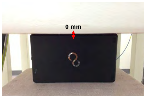
Fig.5 Left side to flat phantom
