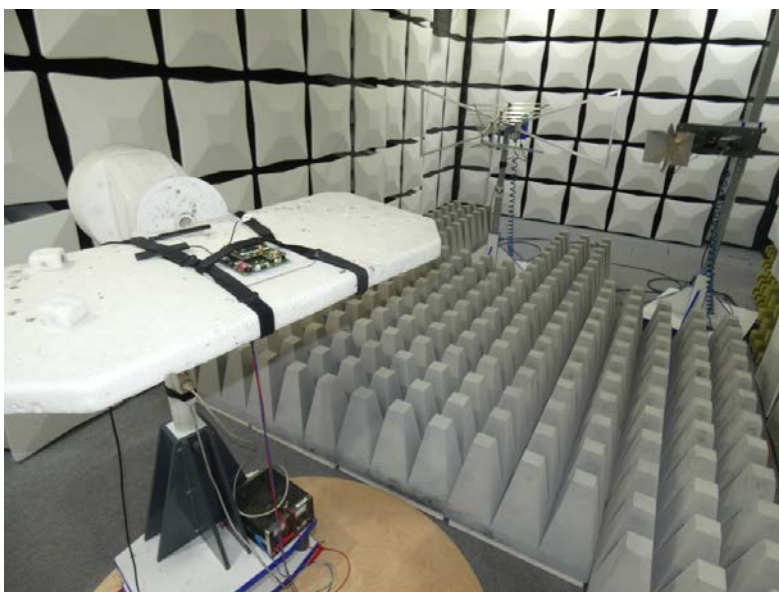
Photo 2: Test setup for radiated measurements (below 1 GHz)
