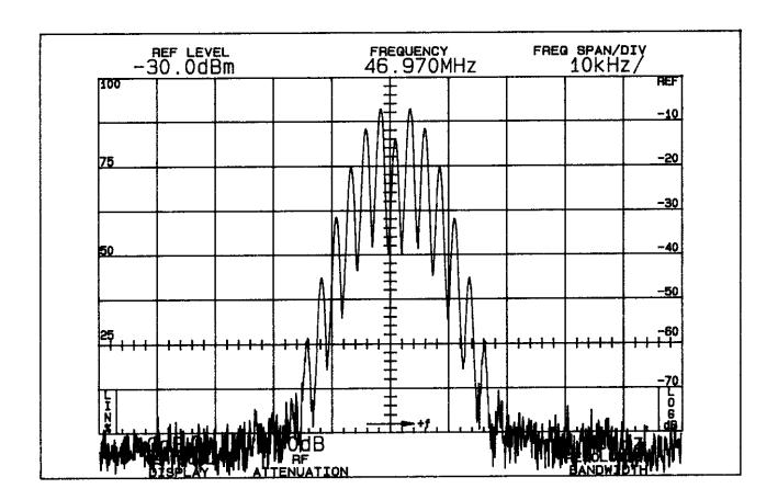
OCCUPIED BANDWIDTH FF777 (B) 2500 Hz Modulation
