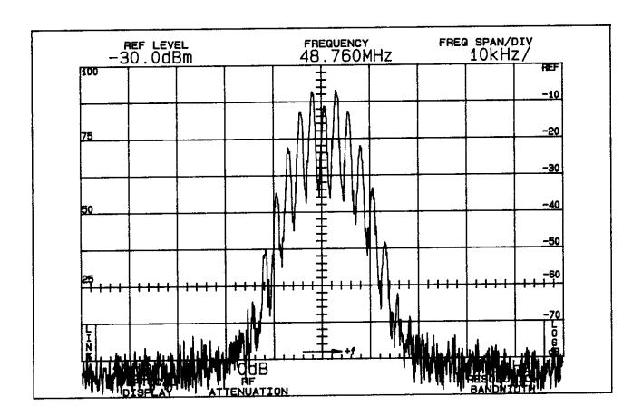
OCCUPIED BANDWIDTH FF777 (H) 2500 Hz Modulation
