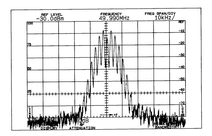
OCCUPIED BANDWIDTH FF777 (H) 2500 Hz Modulation
