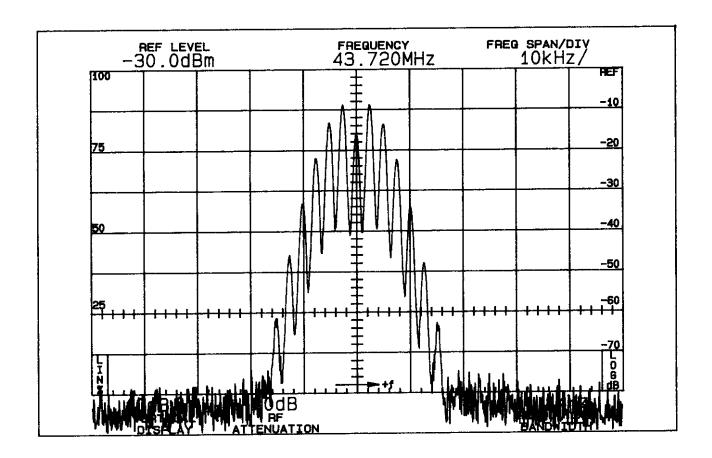
OCCUPIED BANDWIDTH FF777 (B) 2500 Hz Modulation
