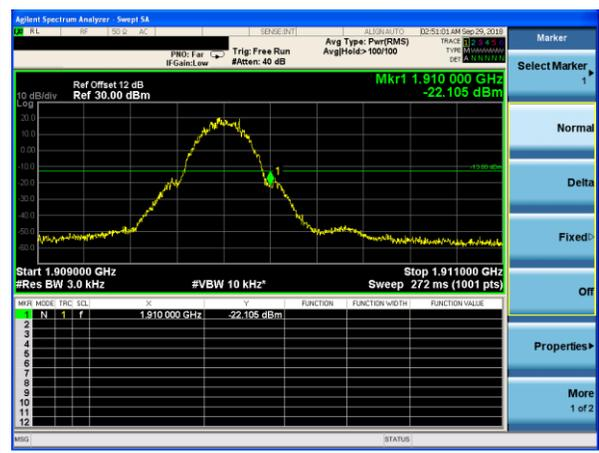
**7.8 CONDUCTED SPURIOUS EMISSION AT ANTENNA TERMINAL**
