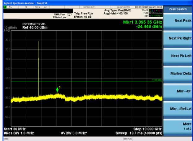
Conducted Emission Transmitting Mode CH 251
