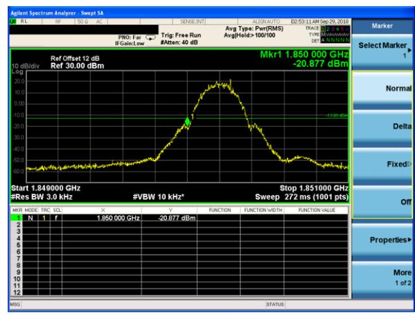
Conducted Band Edge plot on channel 251
