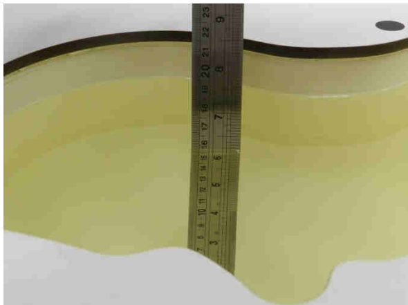
Fig 10.1 Photo of Liquid Height for Head SAR
