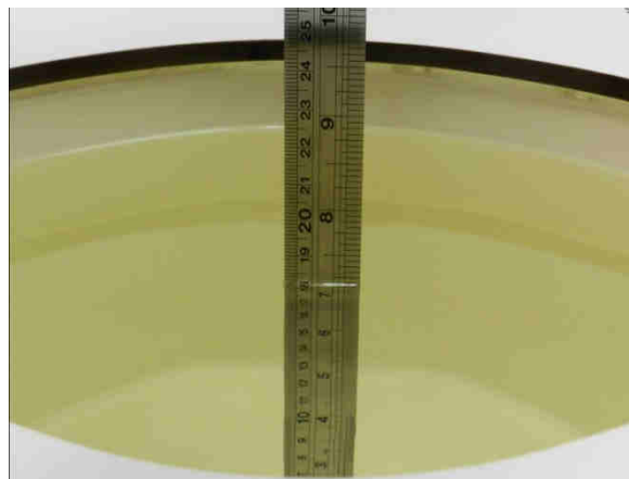
Fig 10.2 Photo of Liquid Height for Body SAR
