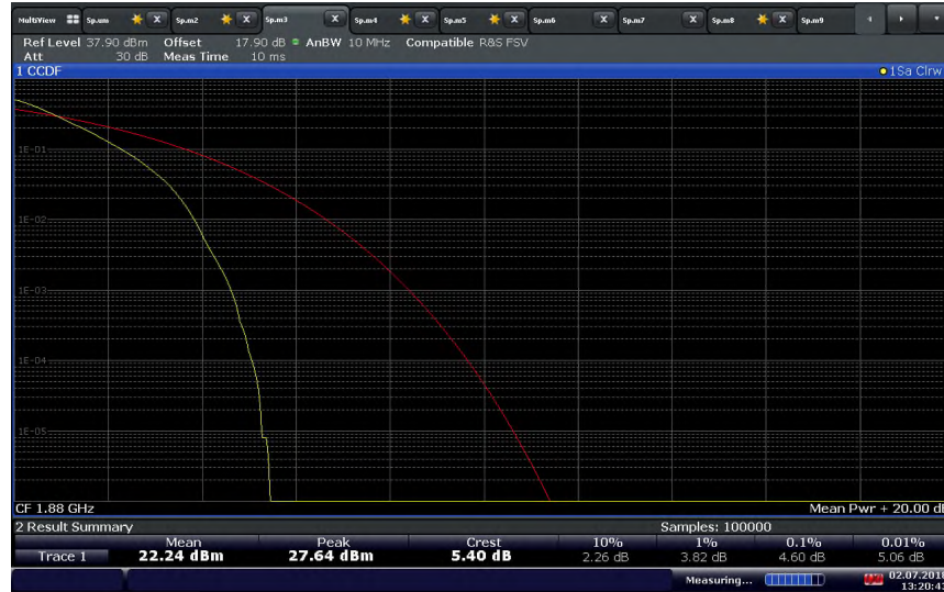
CA_2A-13A_10+10 MHz Bandwidth_PCC_Band 2_1880 MHz_QPSK
