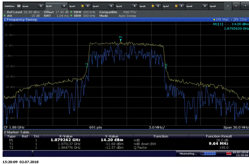
CA_2A-13A_10+10 MHz Bandwidth_PCC_Band 2_1880 MHz_QPSK / 26dB BW
