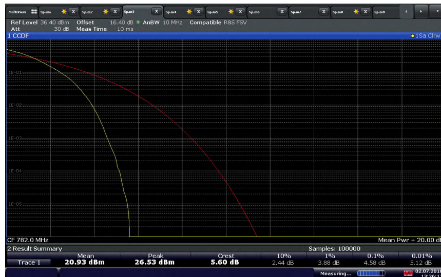
CA_2A-13A_10+10 MHz Bandwidth_SCC_Band 13_782 MHz_QPSK
