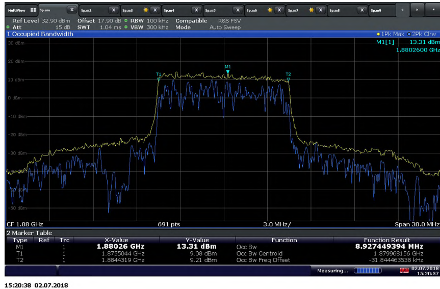
CA_2A-13A_10+10 MHz Bandwidth_PCC_Band 2_1880 MHz_QPSK / 26dB BW
