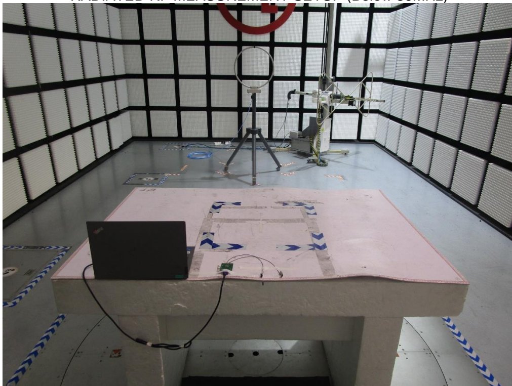
RADIATED RF MEASUREMENT SETUP (Below 30MHz)
