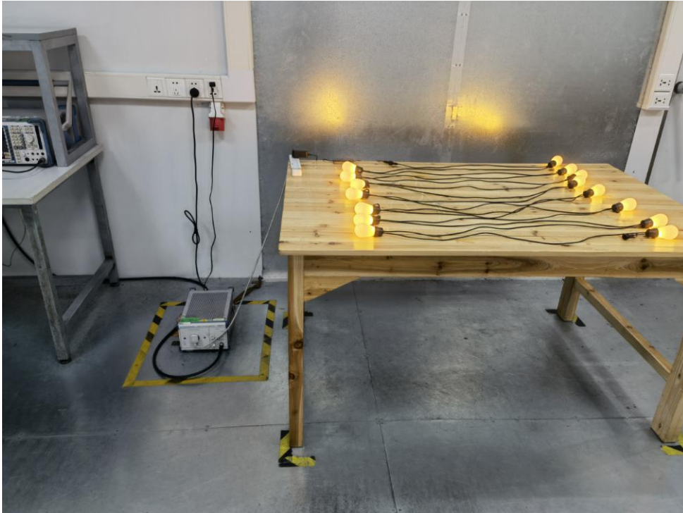
Photo of Conducted Emission Measurement
