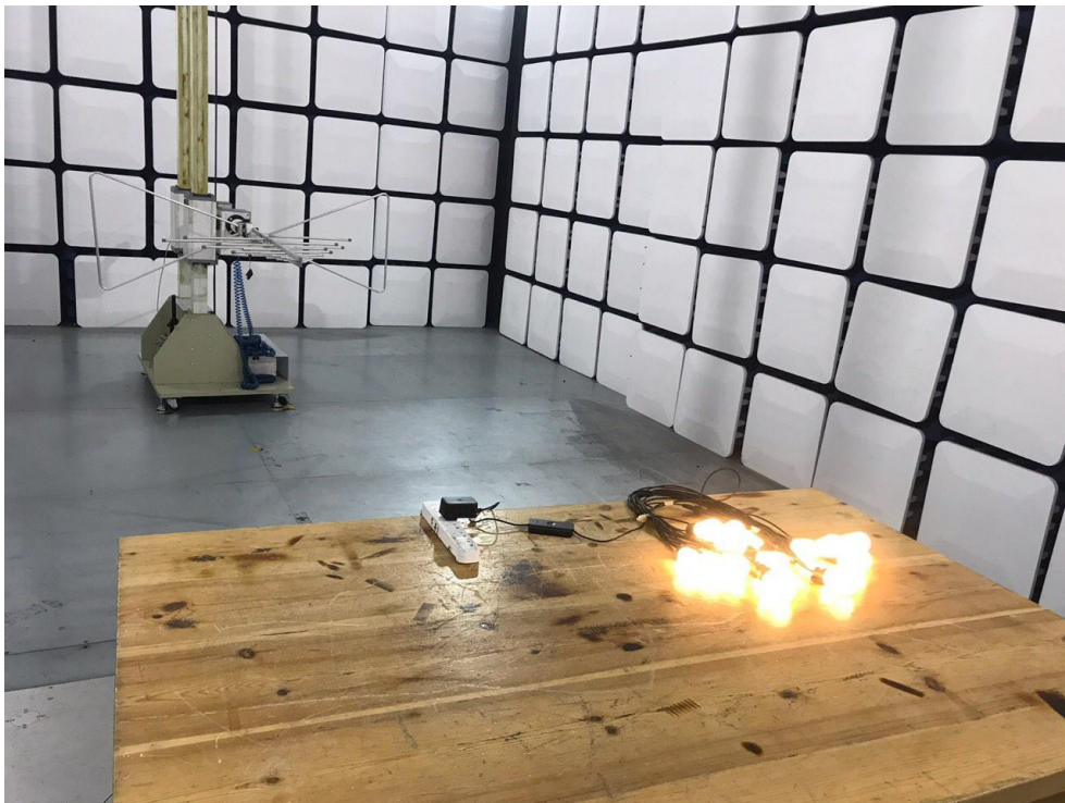
Photo of Radiation Emission Test
