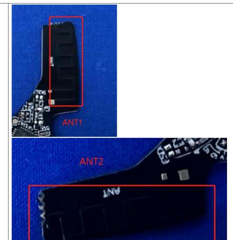
The antenna is PCB antenna.
