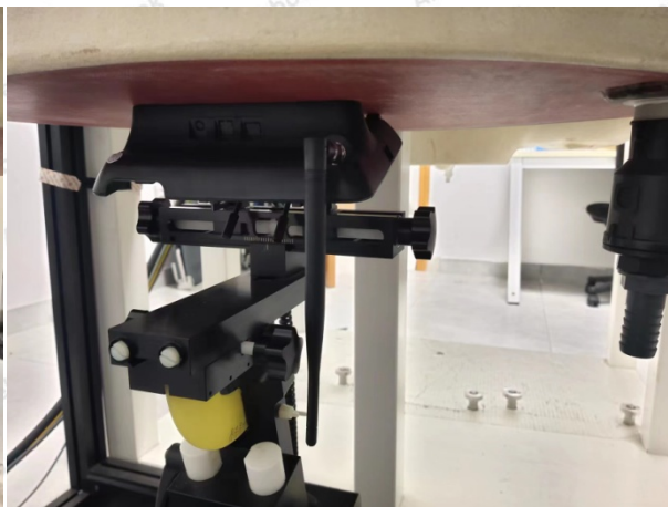
Back with Phantom 0 mm (SAR test with the antenna perpendicular to the device)
