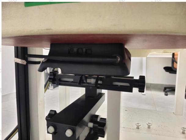
Back with Phantom 0 mm (SAR test with the antenna parallel with the device)
