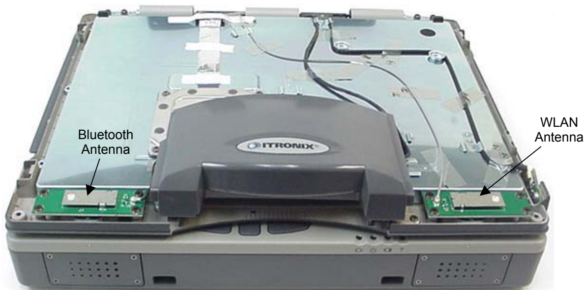
Photograph A-7 - Surface-Mount Antenna Placement
