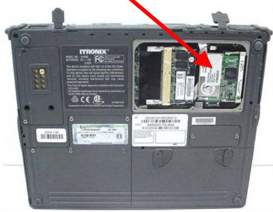
Photograph A-3 - WLAN Mini-PCI Card Location
