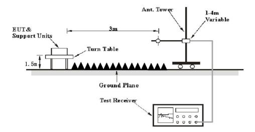
The radiated emission tests were performed in the 3 meters test site, using the setup accordance with the ANSI C63.10-2013 & RSS-Gen. The specification used was the FCC 15.209, and FCC 15.247/RSS-247 limits.
