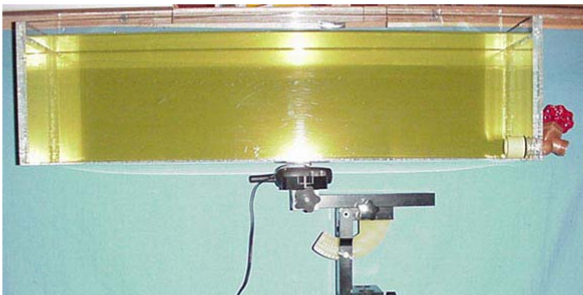
Body-Worn Test Setup Configuration
