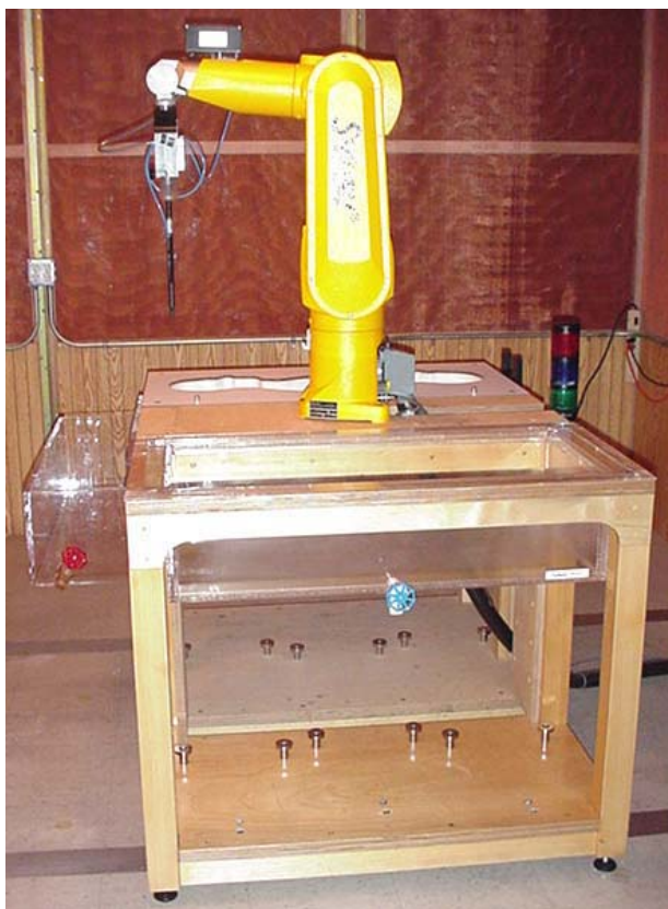
DASY4 SAR Measurement System with validation phantom
