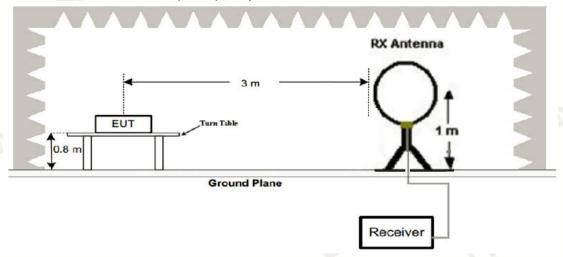
2. Radiated Emission Test-Up Frequency 30MHz~1GHz
