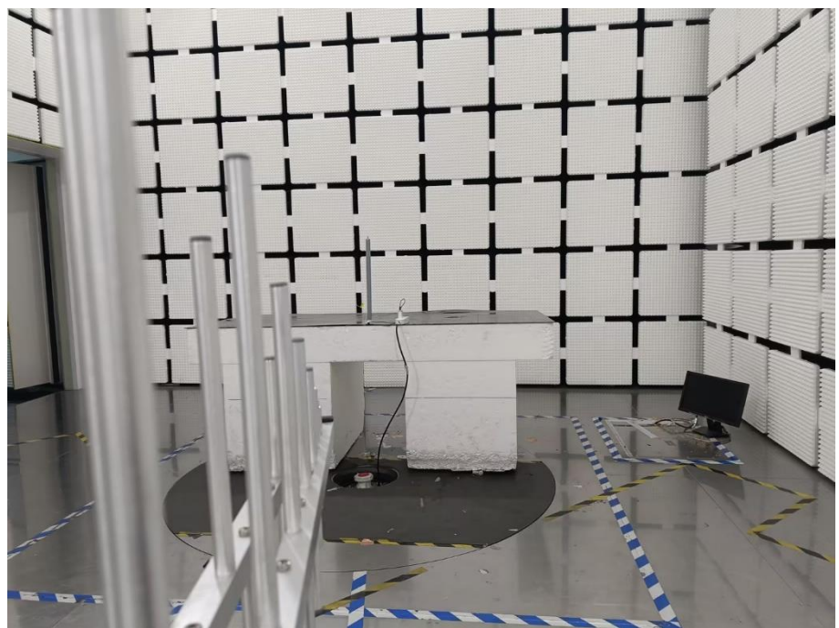
Radiation Emission Test Setup (30MHz to 1GHz)
