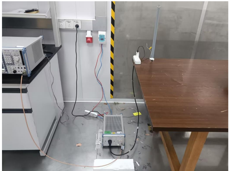
Conducted Emission Test Setup
