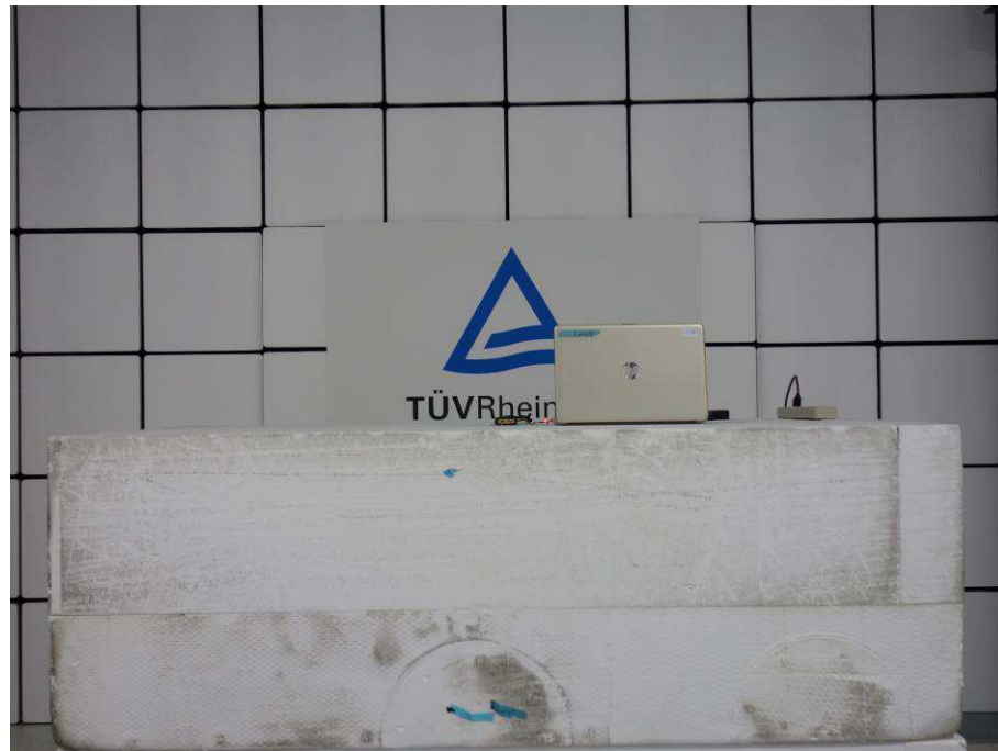
Photograph 2: Set-up for Spurious Emissions (Front View 2)
