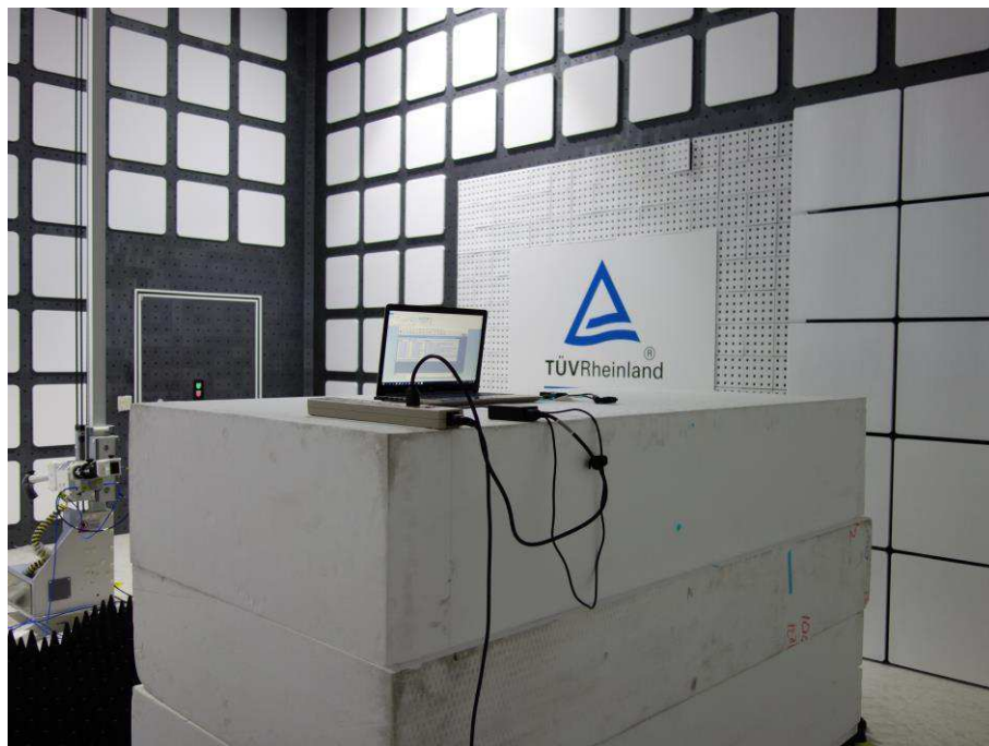
Photograph 4: Set-up for Spurious Emissions (Back View 2)
