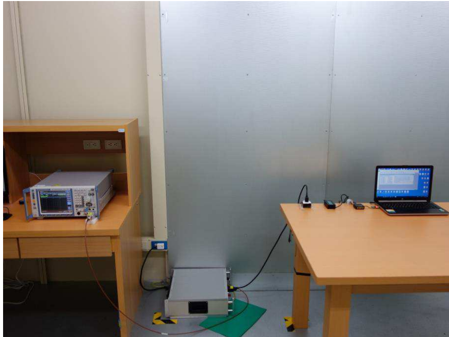
Photograph 9: Set-up for AC Mains Conducted testing (Front View)
