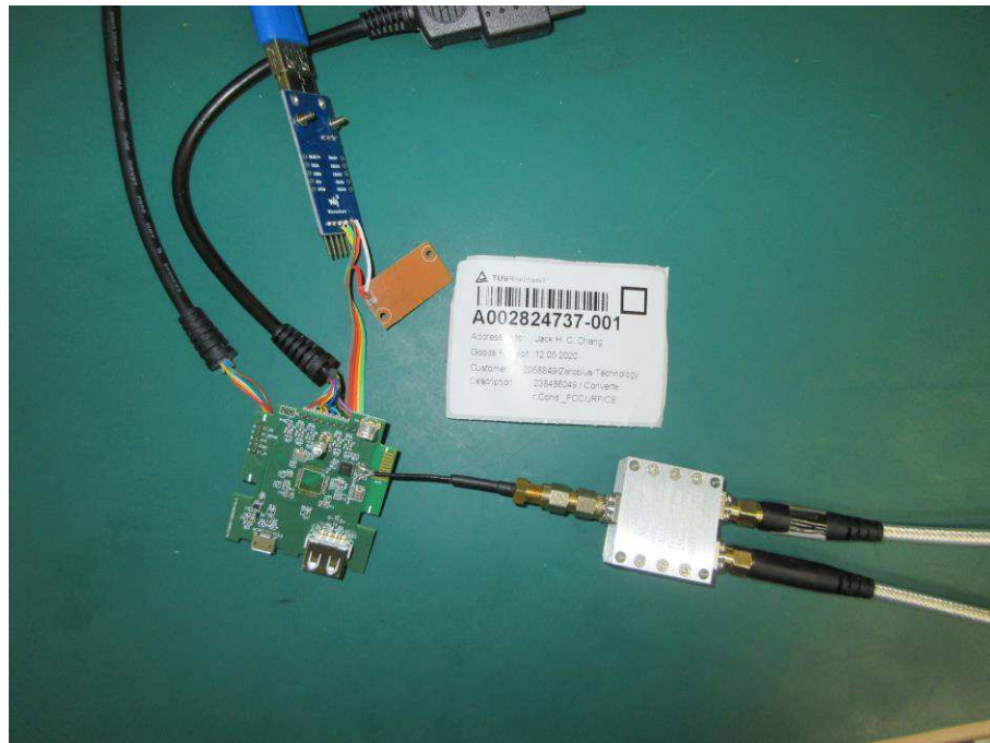
Photograph 8: Set-up for Conducted testing (View 2)
