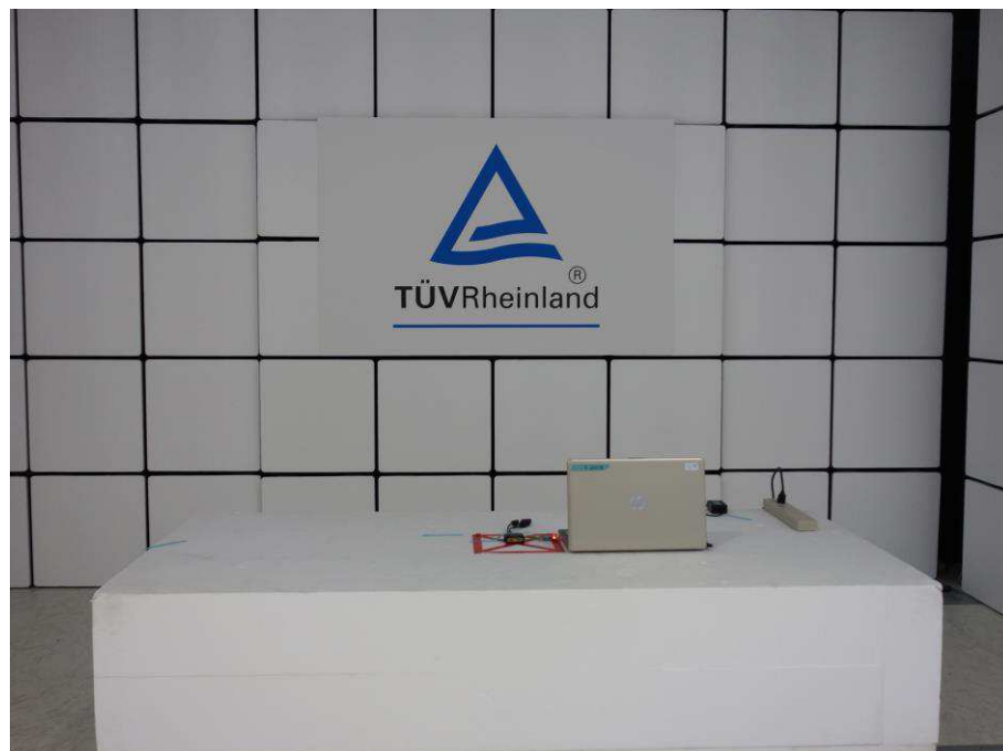
Photograph 2: Set-up for Spurious Emissions (Front View 2)
