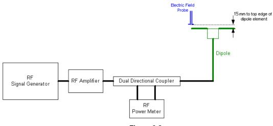
Figure 6-8 System Check Setup
