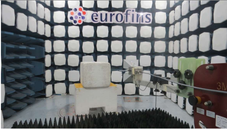
Picture 1 Radiated Emission Test Setup
