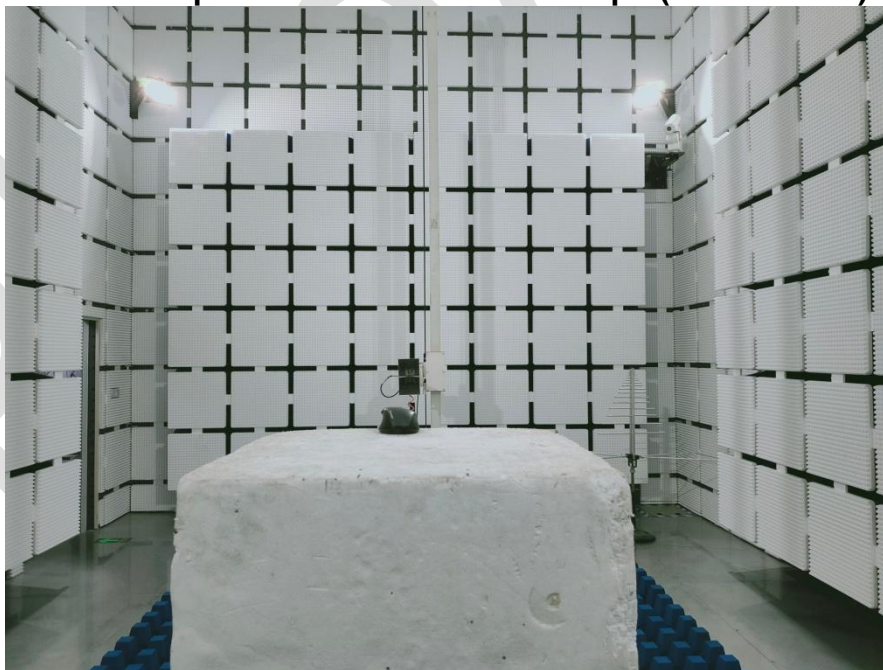
Radiated spurious emission Test Setup-3(Above 1GHz)
