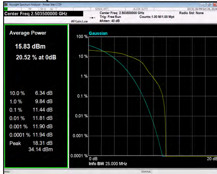
Band41 16QAM BW=15MHz Channel=40620 RB Size=1 Position=#0
