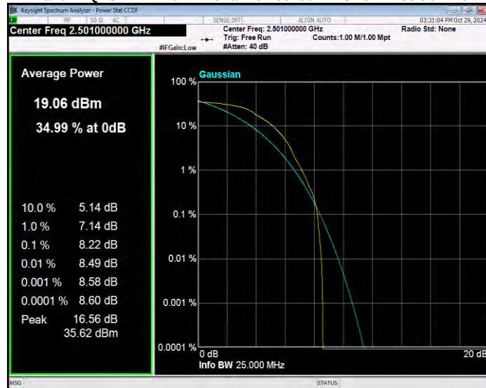
Band41 QPSK BW=10MHz Channel=40620 RB Size=1 Position=#0
