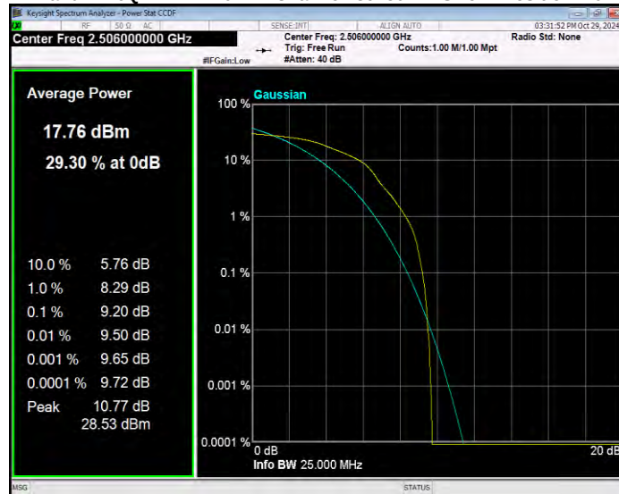
Band41 16QAM BW=20MHz Channel=40620 RB Size=1 Position=#0
