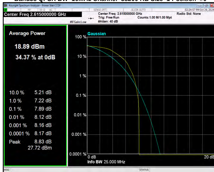
Band38 QPSK BW=15MHz Channel=37825 RB Size=1 Position=#0
