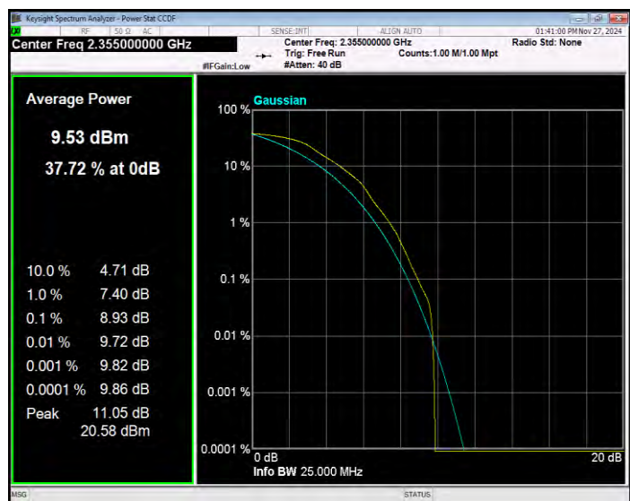
Band40(2350-2360) QPSK BW=5MHz Channel=39225 RB Size=1 Position=#0
