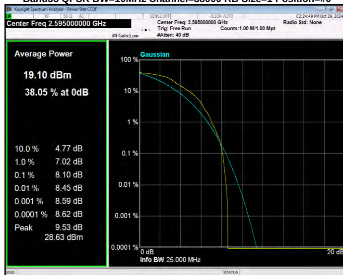
Band38 QPSK BW=10MHz Channel=38200 RB Size=1 Position=#0
