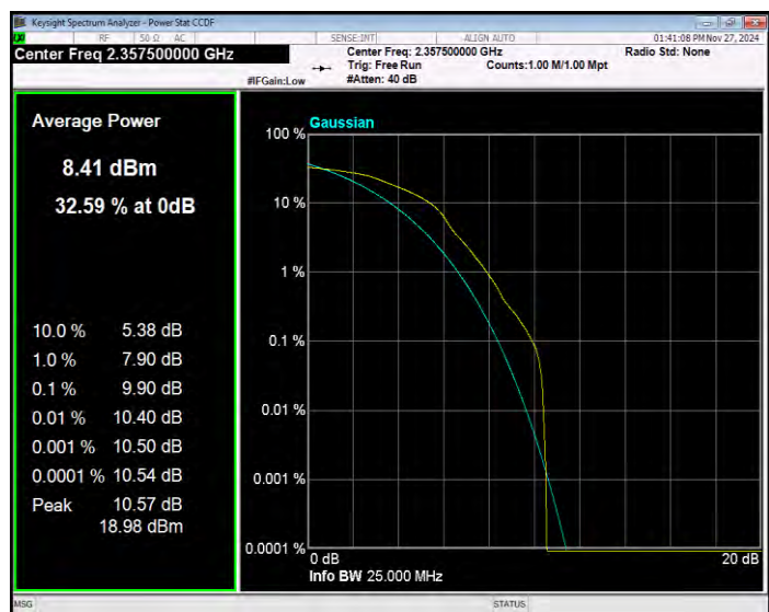
Band40(2350-2360) QPSK BW=10MHz Channel=39200 RB Size=1 Position=#0
