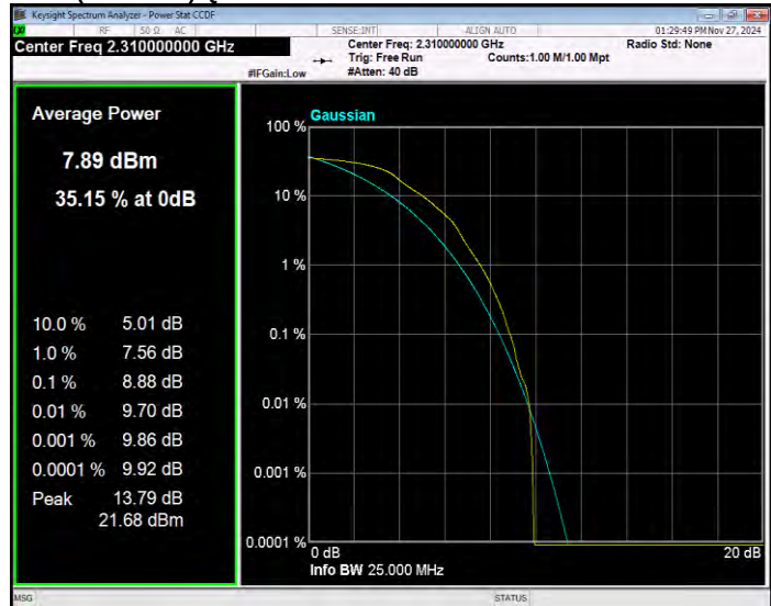
Band40(2305-2315) QPSK BW=5MHz Channel=38775 RB Size=1 Position=#0
