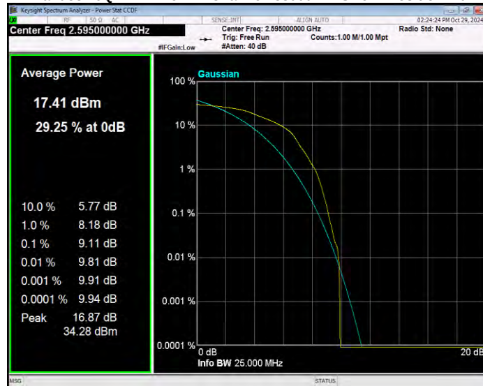
Band38 16QAM BW=5MHz Channel=38225 RB Size=1 Position=#0
