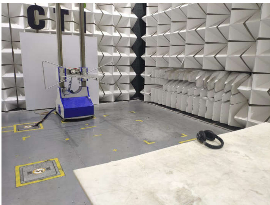
Radiated spurious emission Test Setup-2(Below 1GHz)
