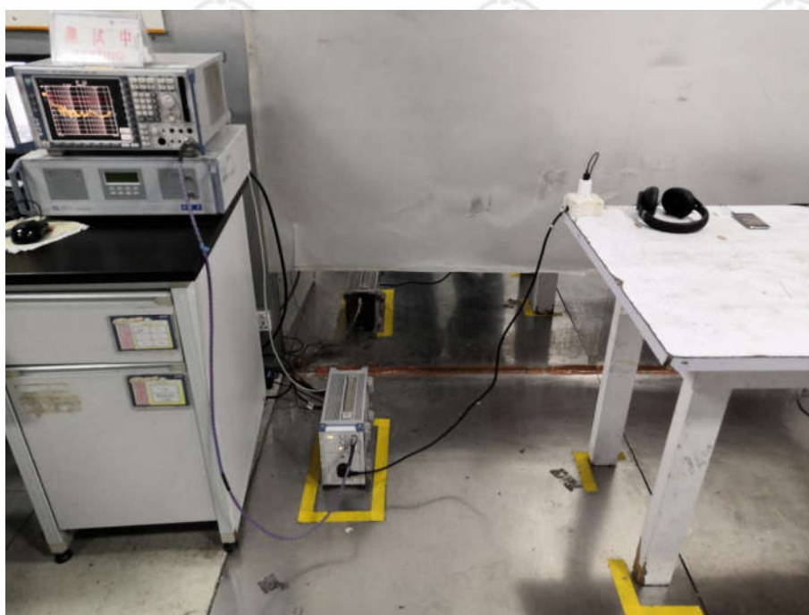
Conducted Emissions Test Setup
