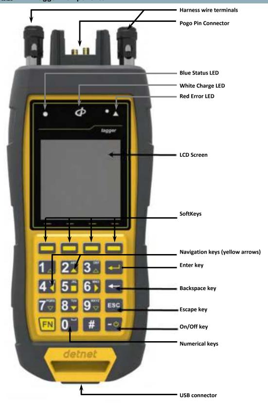
Figure 4: CE4 Tagger Component Identification
