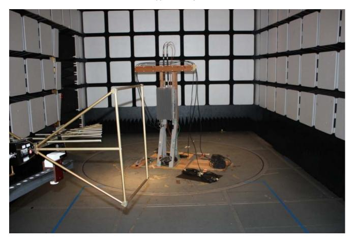
TEST: **Measurement of Radiated Spurious Emissions**
