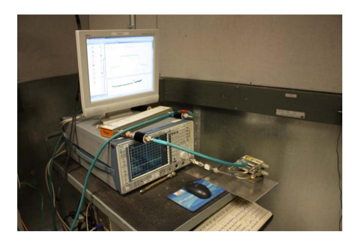
**TEST:** Measurement of Radiated Spurious Emissions
