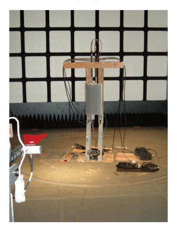
**TEST:** Measurement of Radiated Spurious Emissions
