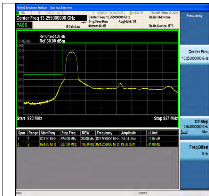
Band5 3MHz 16QAM 20415 1RB#0
