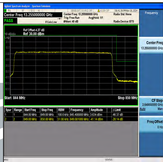
Band5 5MHz 16QAM 20625 25RB#0
