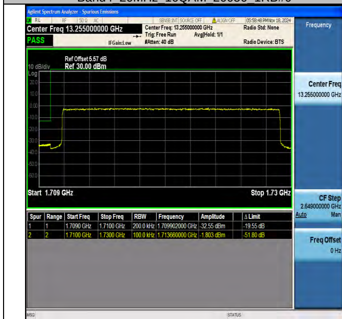
Band4 20MHz 16QAM 20050 100RB#0
