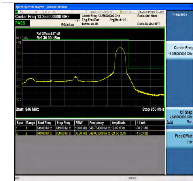
Band5 3MHz 16QAM 20635 1RB#14
