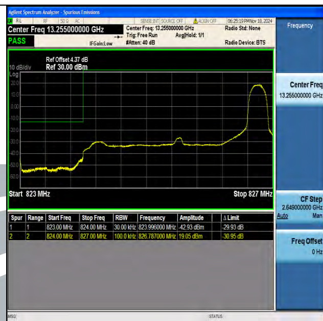
Band5 3MHz 16QAM 20415 1RB#14
