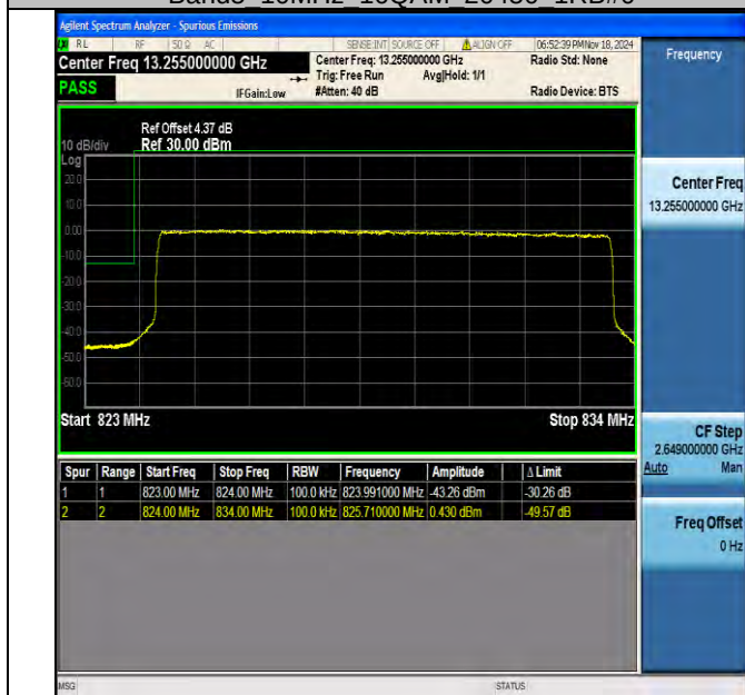
Band5 10MHz 16QAM 20450 50RB#0
