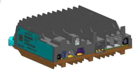
During all test the EUT was supplied with 13.5 V DC via a laboratory power supply. During the tests, a USB connection was established to the EUT via USB-2-optic converter. All relevant HF parameters could be set with a Laptop.
