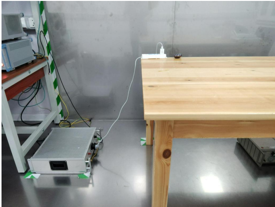
Conducted Emission at AC power line
