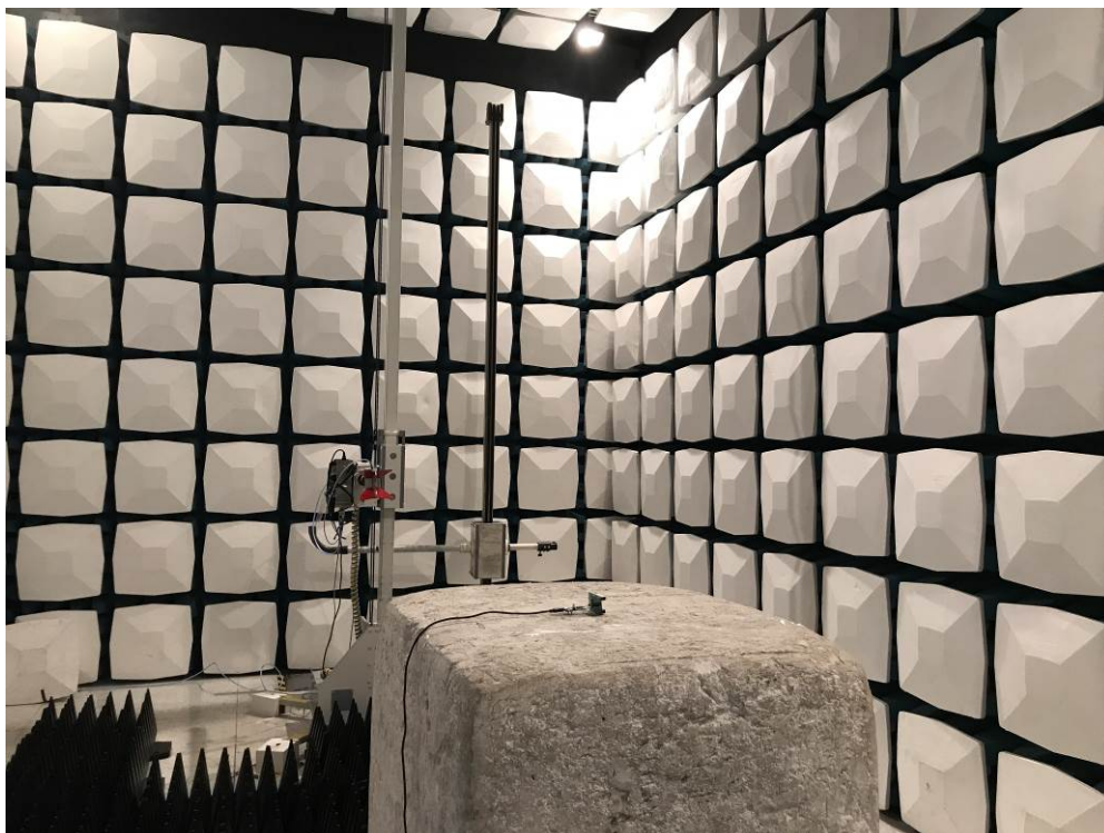
Description: Radiated Emission Test Setup for 1~18GHz
