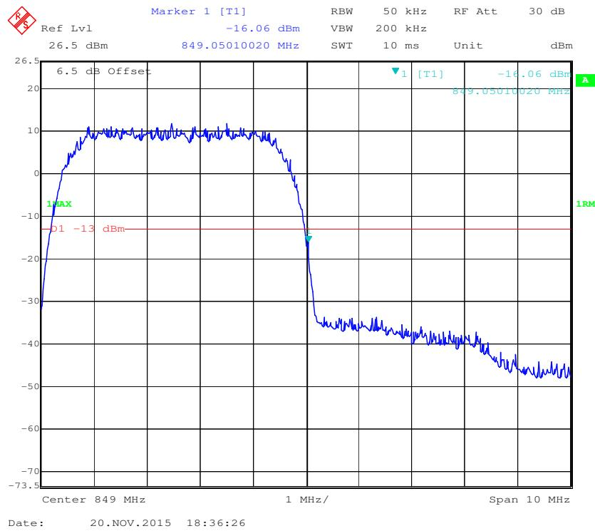
**Cellular Band, Left Band Edge for HSDPA (16QAM) Mode**
