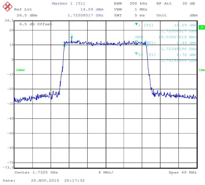
**16-QAM (20.0 MHz) - 99% Occupied Bandwidth, Middle channel**
