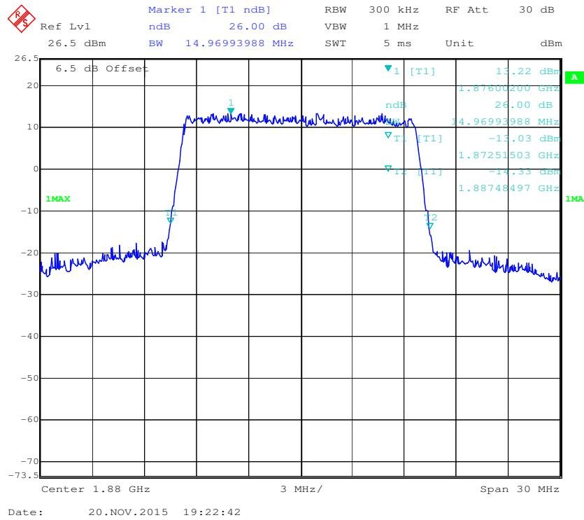
**QPSK (20.0 MHz) - 26 dB Bandwidth, Middle channel**
