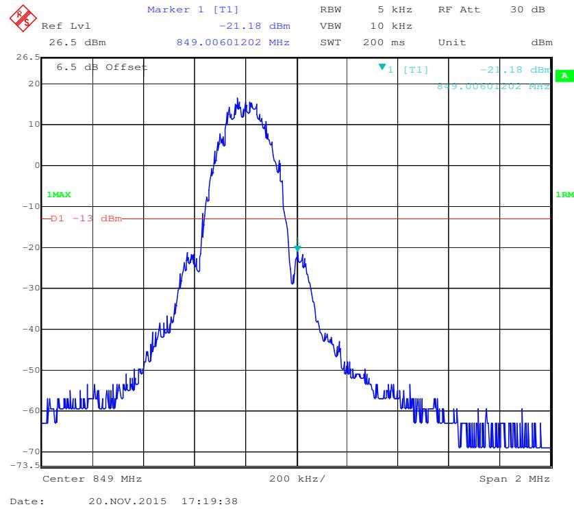
**Cellular Band, Left Band Edge for WCDMA (BPSK) Mode**
