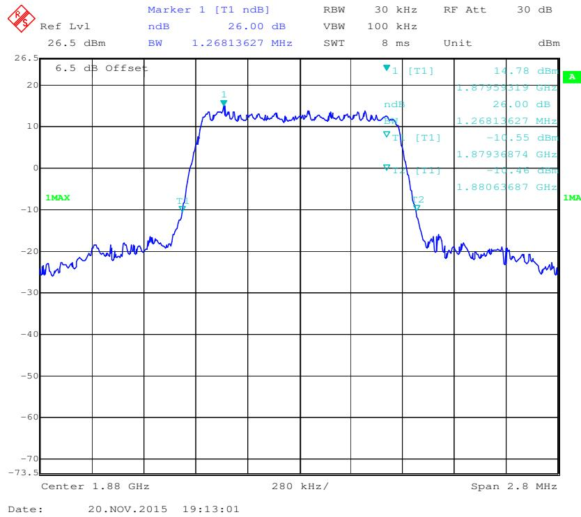
**QPSK (3.0 MHz) - 26 dB Bandwidth, Middle channel**
