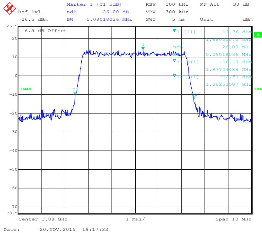
**QPSK (10.0 MHz) - 26 dB Bandwidth, Middle channel**
