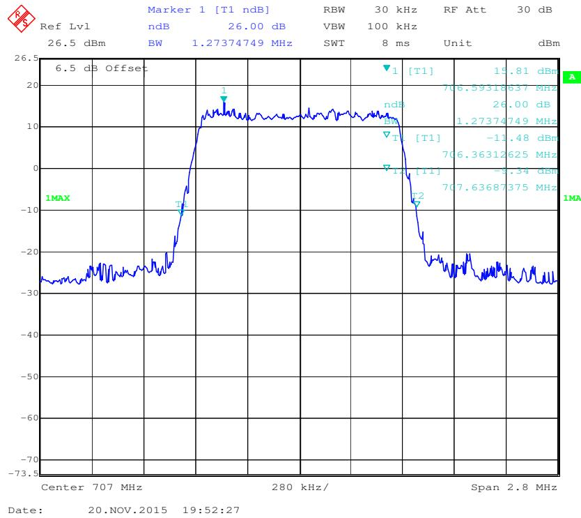
**QPSK (3.0MHz) - 26 dB Bandwidth, Middle channel**
