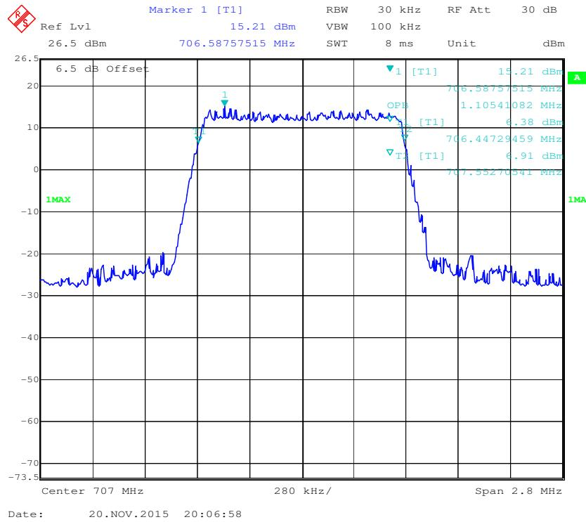
**QPSK (3.0 MHz) - 99% Occupied Bandwidth, Middle channel**
