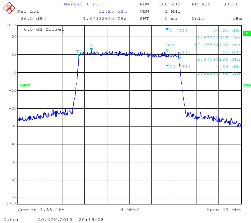
**QPSK (1.4 MHz) - 26 dB Bandwidth, Middle channel**
