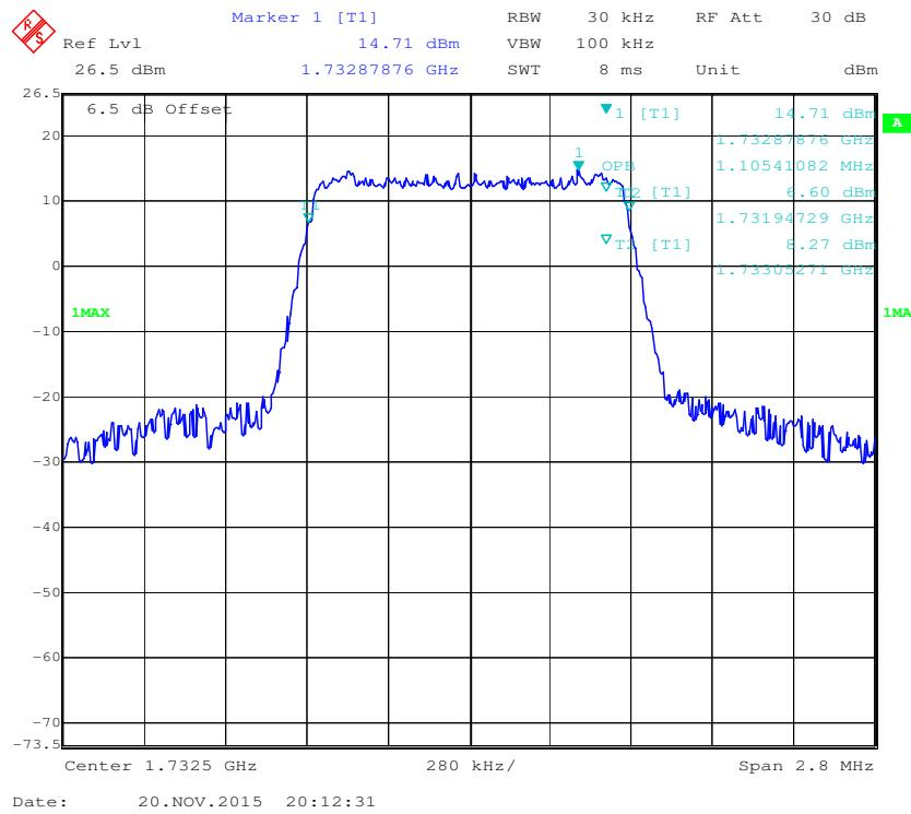
**QPSK (3.0 MHz) - 99% Occupied Bandwidth, Middle channel**
