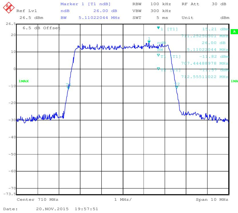
**16-QAM (5.0 MHz) - 26 dB Bandwidth, Middle channel**
