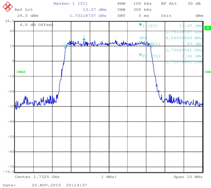
**QPSK (10.0 MHz) - 99% Occupied Bandwidth, Middle channel**
