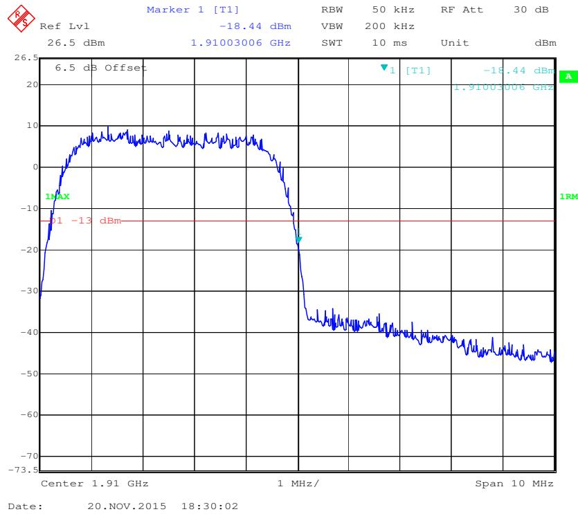
**AWS Band, Left Band Edge for WCDMA (BPSK) Mode**
