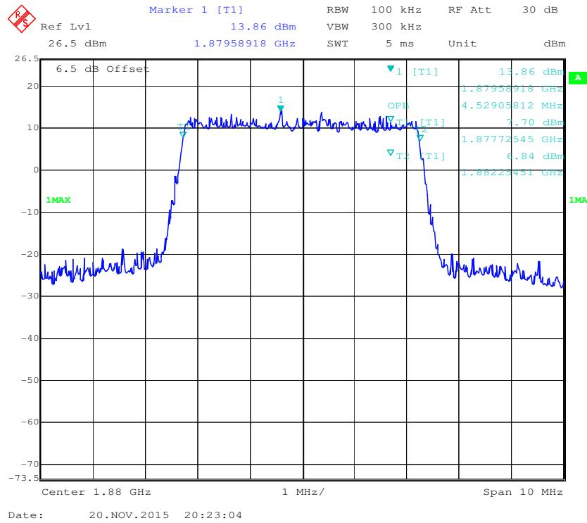
**QPSK (10.0 MHz) - 99% Occupied Bandwidth, Middle channel**
