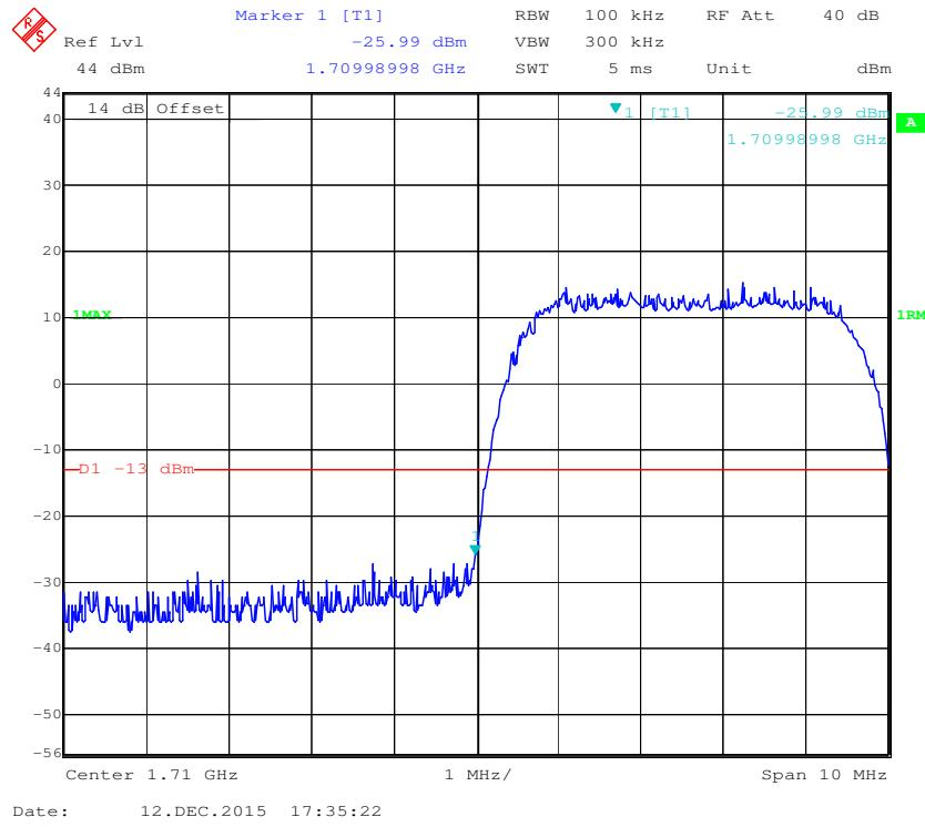
**AWS Band, Right Band Edge for HSDPA (16QAM) Mode**
