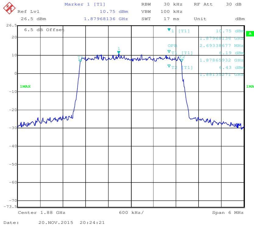
**QPSK (5.0 MHz) - 99% Occupied Bandwidth, Middle channel**
