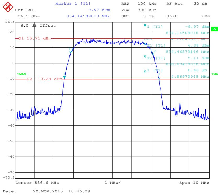
**PCS Band (Part 24E)****99% Occupied &26 dB Emissions Bandwidth for GSM (GMSK) Mode**
