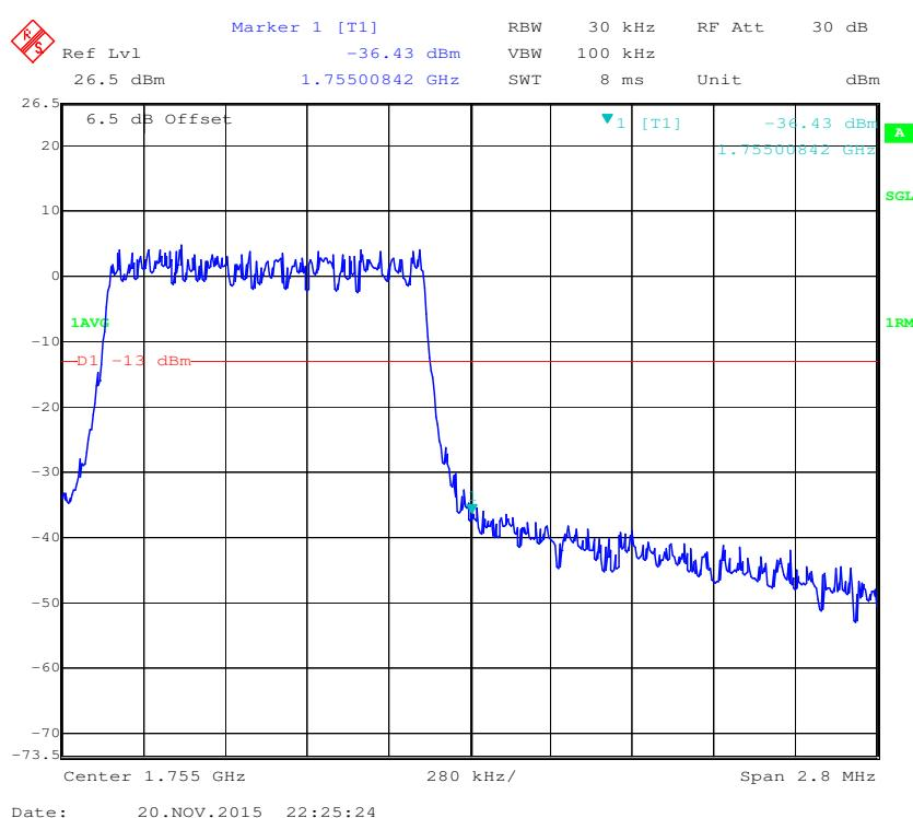
**16-QAM (1.4 MHz, FULL RB) - Left Band Edge**
