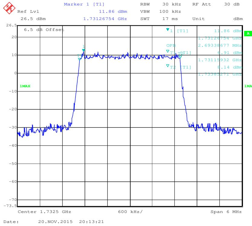
**16-QAM (3.0 MHz) - 99% Occupied Bandwidth, Middle channel**
