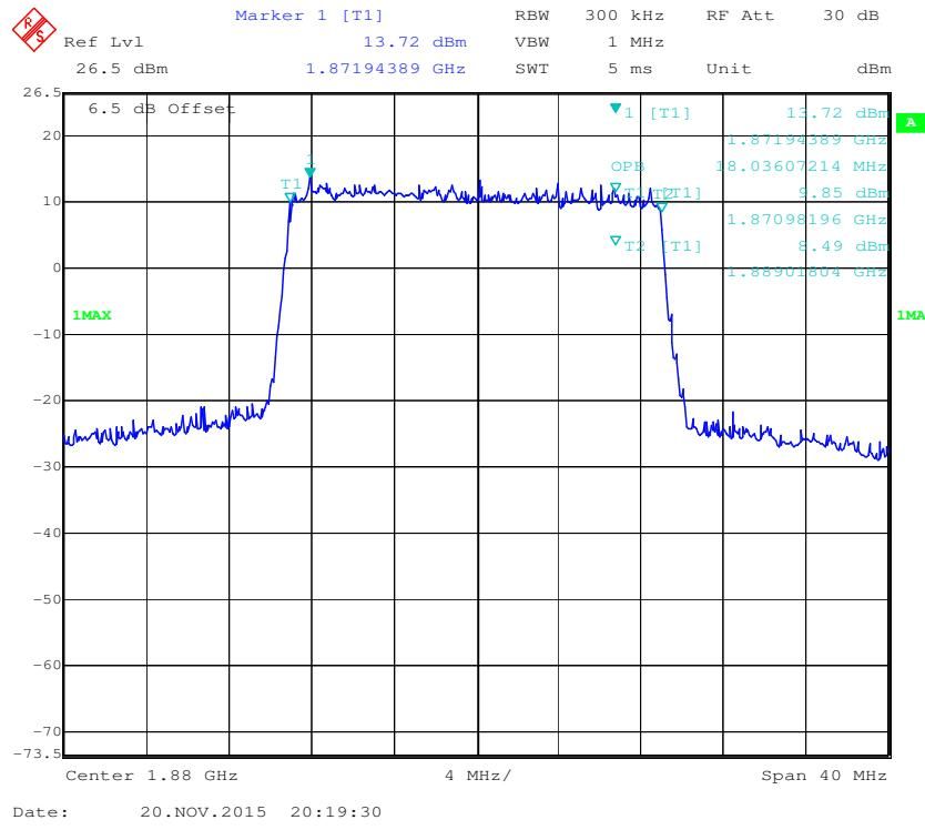
**16-QAM (20.0 MHz) - 99% Occupied Bandwidth, Middle channel**
