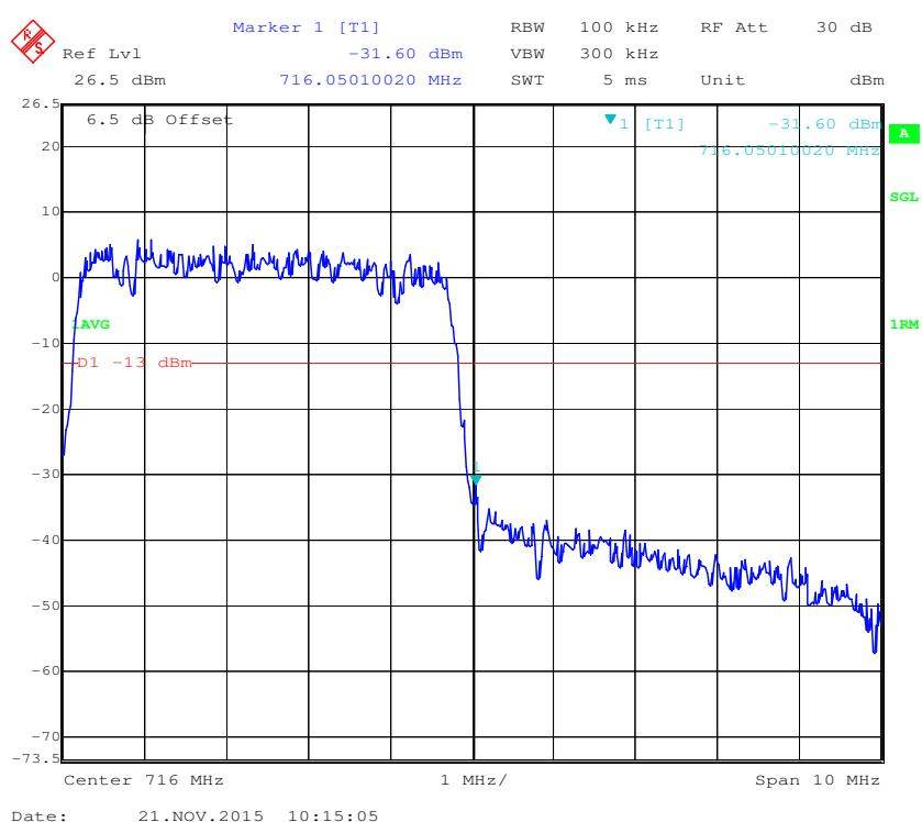
**16-QAM (5.0 MHz, FULL RB) - Left Band Edge**
