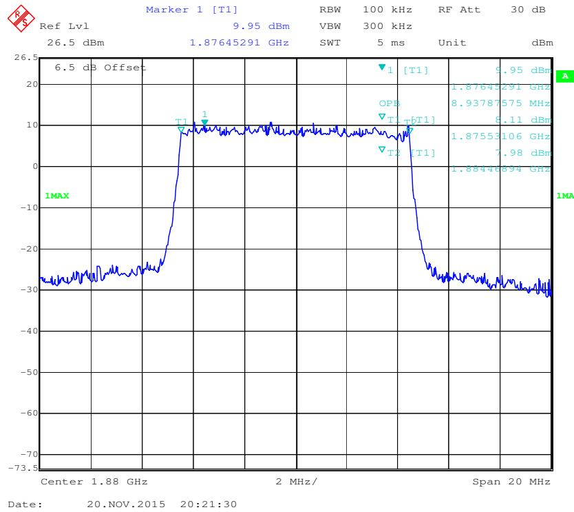
**QPSK (15.0 MHz) - 99% Occupied Bandwidth, Middle channel**
