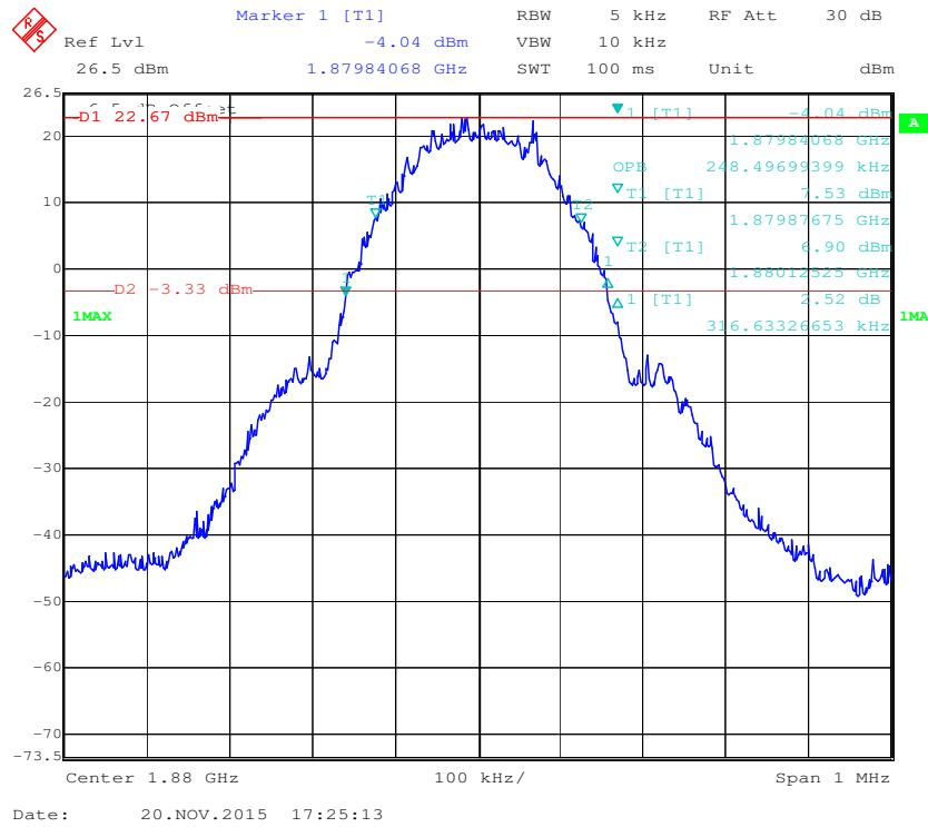
**99% Occupied &26 dB Emissions Bandwidth for EGPRS Mode**
