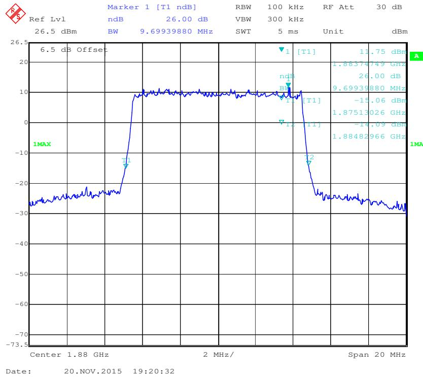
**QPSK (15.0 MHz) - 26 dB Bandwidth, Middle channel**
