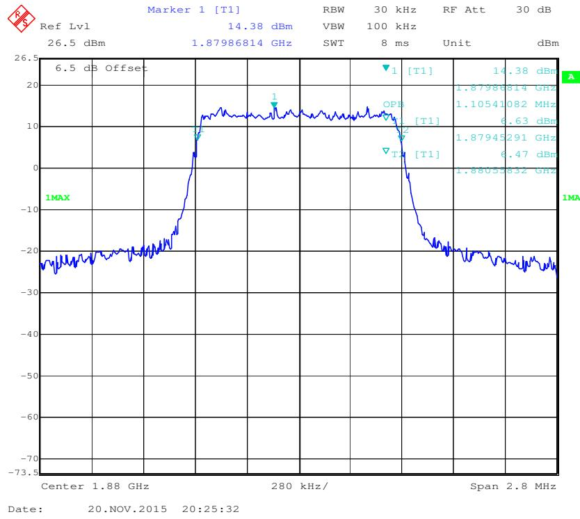
**16-QAM (1.4 MHz) - 99% Occupied Bandwidth, Middle channel**
