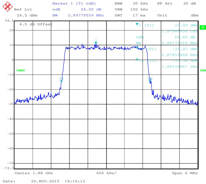
**QPSK (5.0 MHz) - 26 dB Bandwidth, Middle channel**
