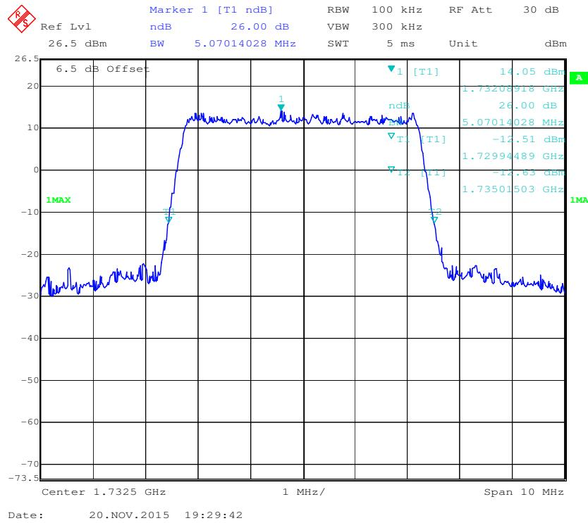
**QPSK (10.0 MHz) - 26 dB Bandwidth, Middle channel**
