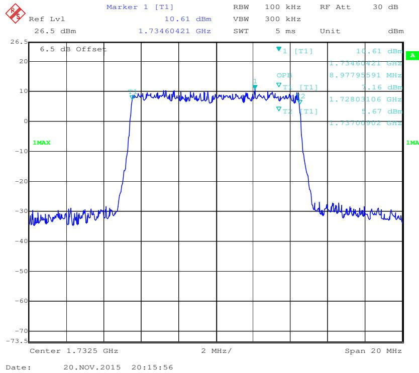
**QPSK (15.0 MHz) - 99% Occupied Bandwidth, Middle channel**
