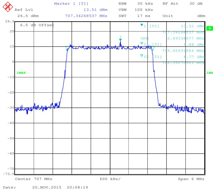
**QPSK (5.0 MHz) - 99% Occupied Bandwidth, Middle channel**
