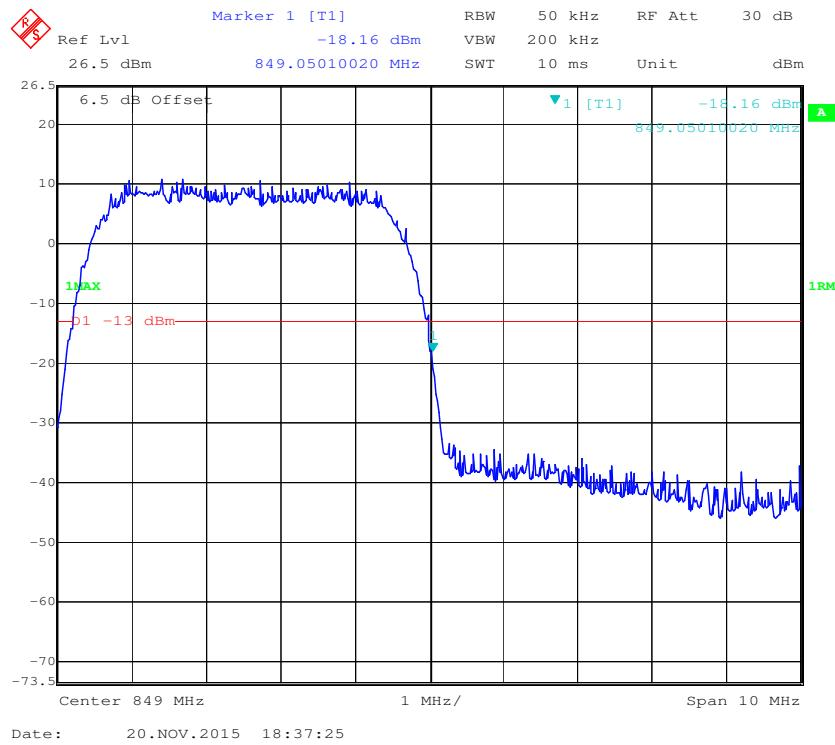
**PCS Band, Left Band Edge for GSM (GMSK) Mode**
