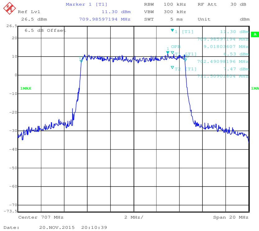
**QPSK (1.4 MHz) - 26 dB Bandwidth, Middle channel**
