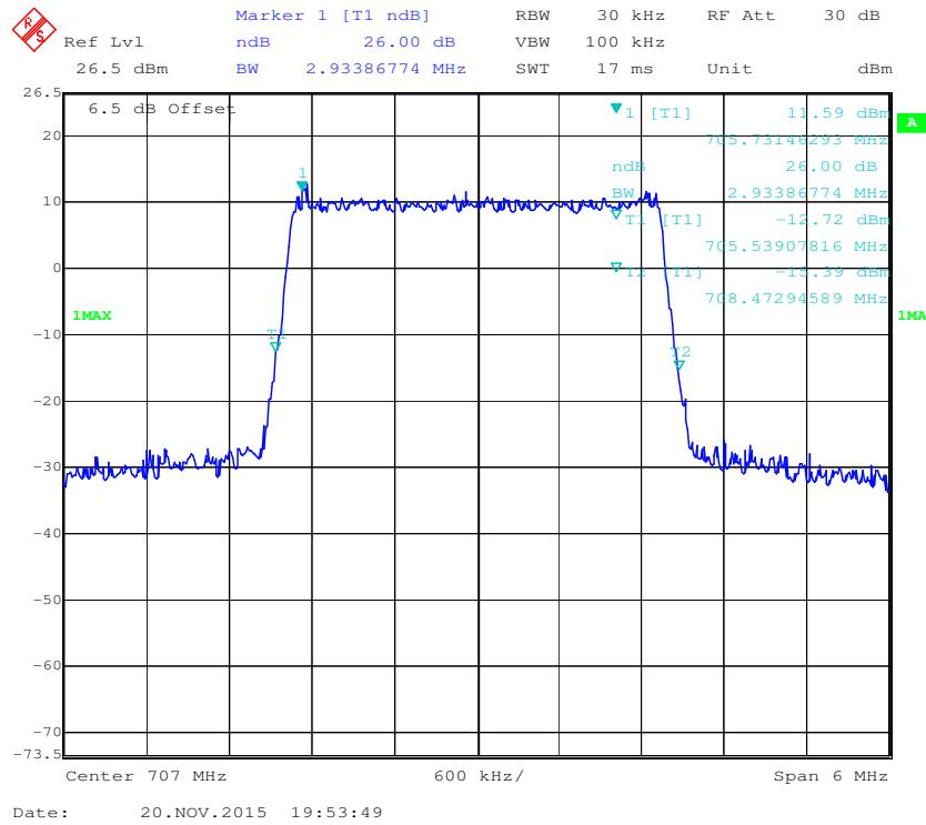
**QPSK (5.0 MHz) - 26 dB Bandwidth, Middle channel**
