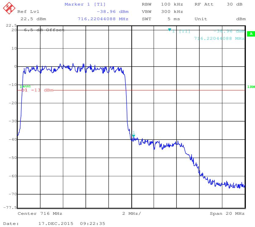
**Band 17:****QPSK (5.0 MHz, FULL RB) - Left Band Edge**
