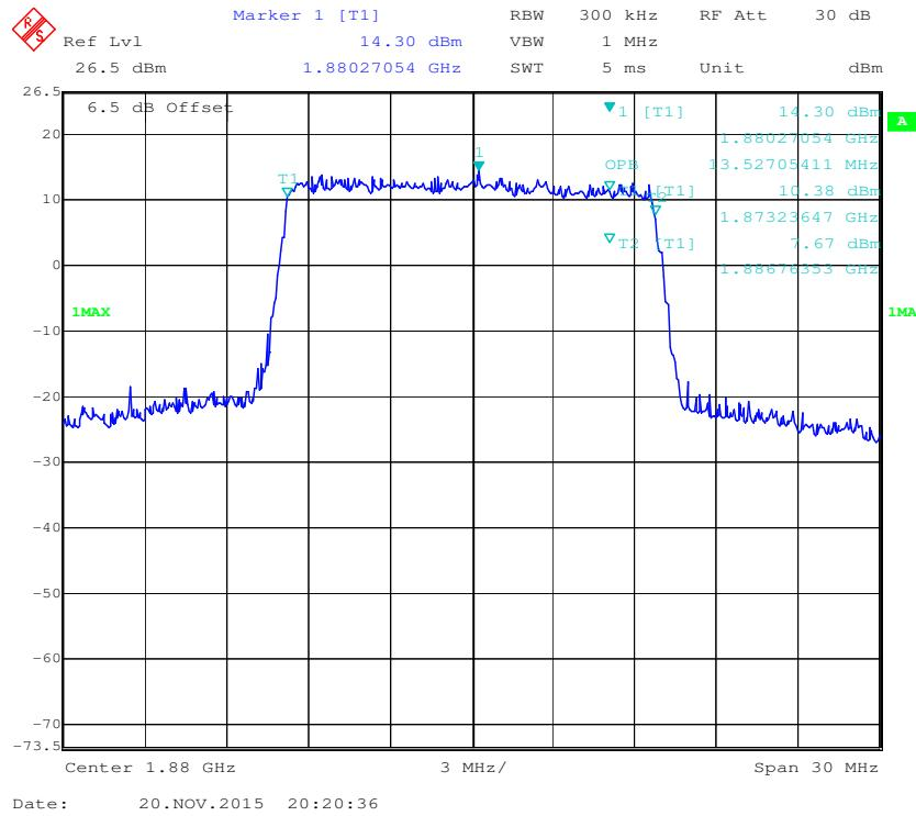
**QPSK (20.0 MHz) - 99% Occupied Bandwidth, Middle channel**
