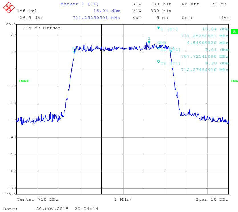
**QPSK (10.0 MHz) - 99% Occupied Bandwidth, Middle channel**
