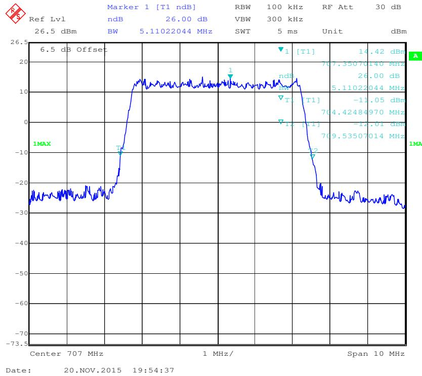
**QPSK (10.0 MHz) - 26 dB Bandwidth, Middle channel**
