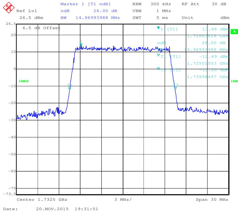
**16-QAM (15.0 MHz) - 26 dB Bandwidth, Middle channel**
