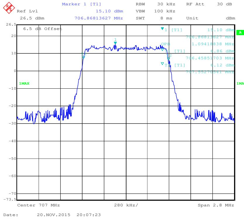
**16-QAM (1.4 MHz) - 99% Occupied Bandwidth, Middle channel**
