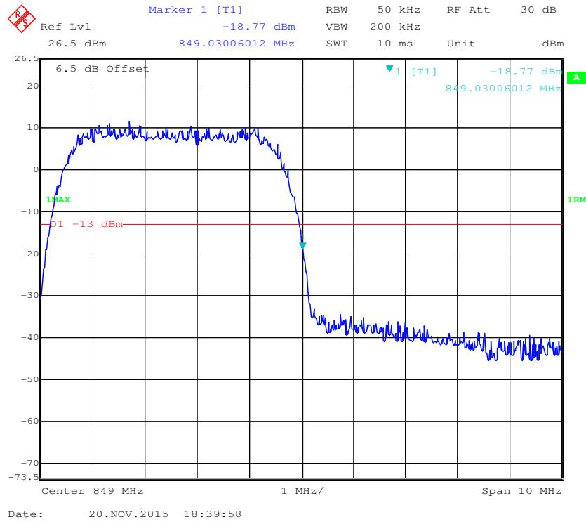
**Cellular Band, Left Band Edge for HSUPA (BPSK) Mode**
