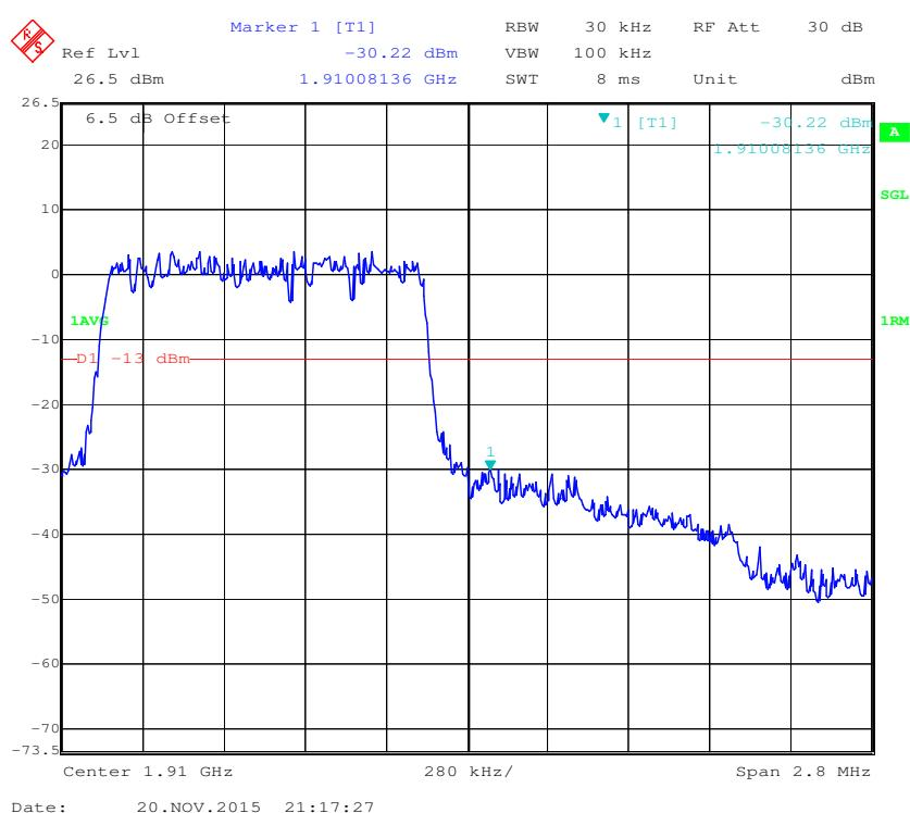
**16-QAM (1.4 MHz, FULL RB) - Left Band Edge**
