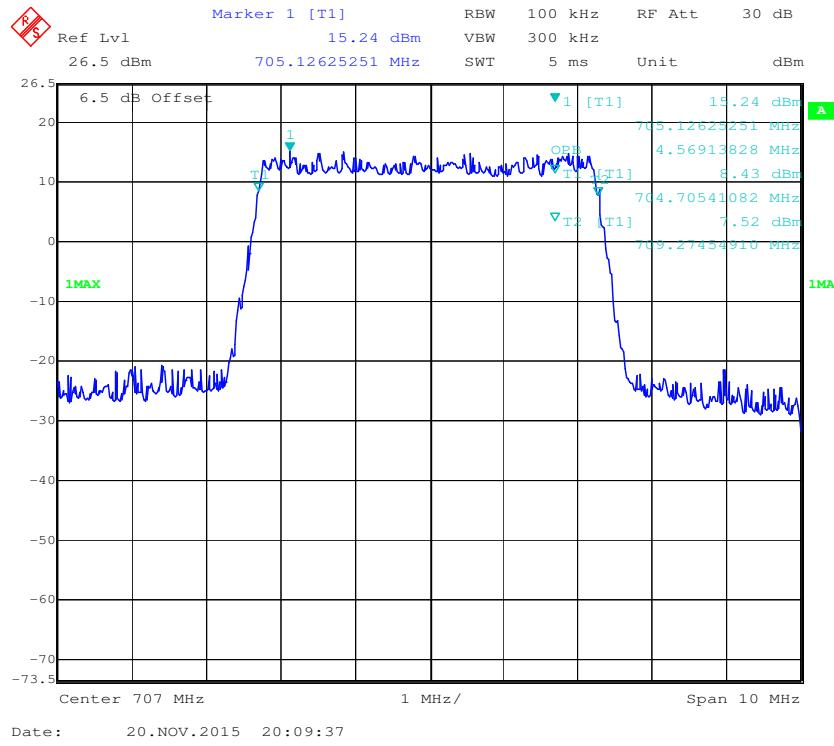
**16-QAM (5.0 MHz) - 99% Occupied Bandwidth, Middle channel**
