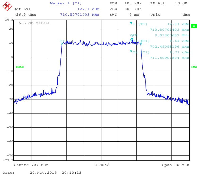
**16-QAM (10.0MHz) - 99% Occupied Bandwidth, Middle channel**
