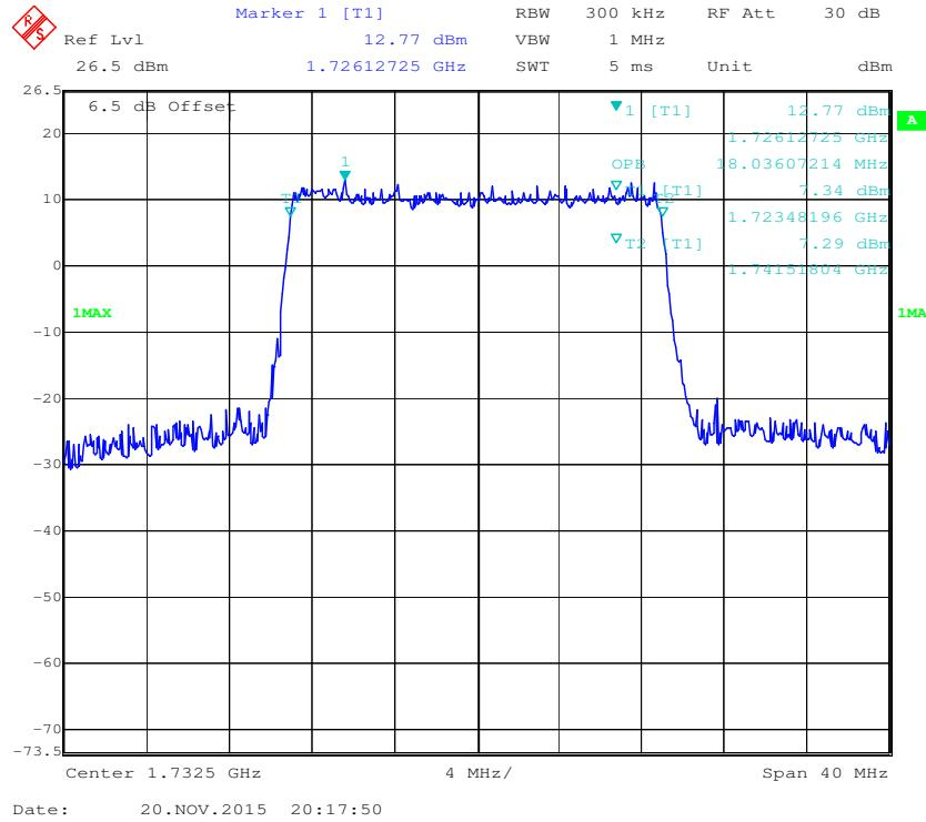
**QPSK (1.4 MHz) - 26 dB Bandwidth, Middle channel**
