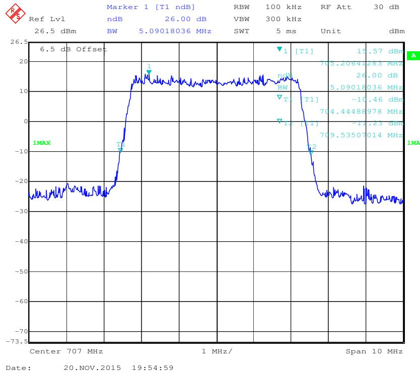
**16-QAM (5.0 MHz) - 26 dB Bandwidth, Middle channel**
