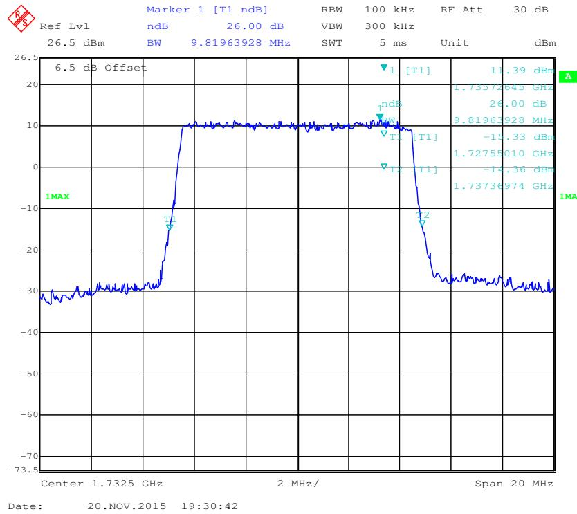
**QPSK (15.0 MHz) - 26 dB Bandwidth, Middle channel**
