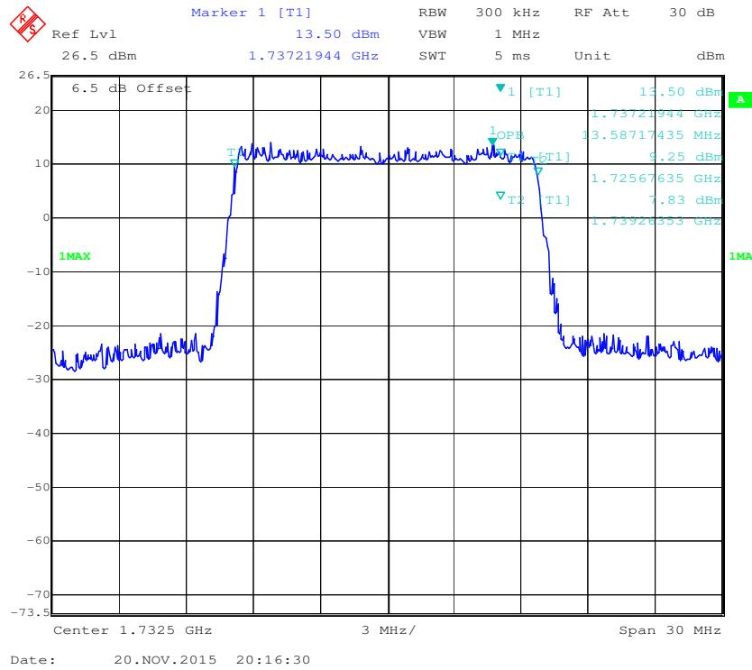
**QPSK (20.0 MHz) - 99% Occupied Bandwidth, Middle channel**
