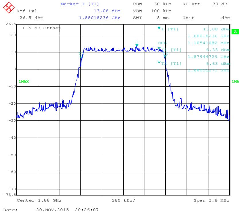
**QPSK (3.0 MHz) - 99% Occupied Bandwidth, Middle channel**
