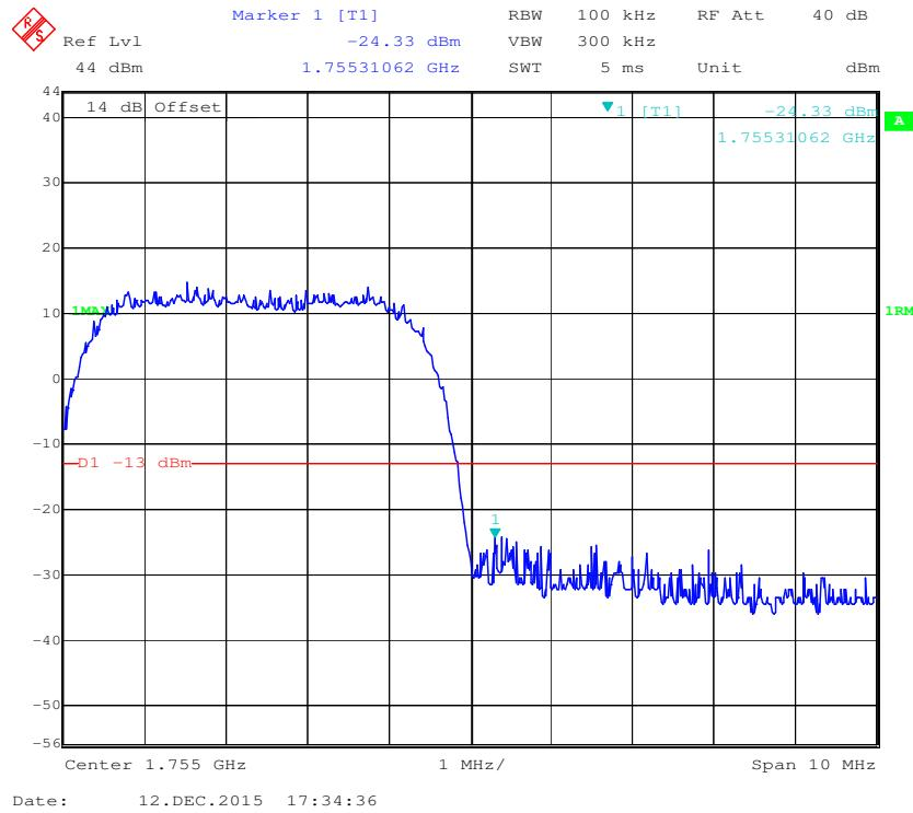
**AWS Band, Left Band Edge for HSUPA (BPSK) Mode**
