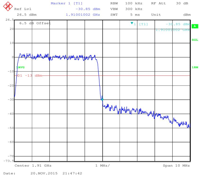
**16-QAM (5.0 MHz, FULL RB) - Left Band Edge**
