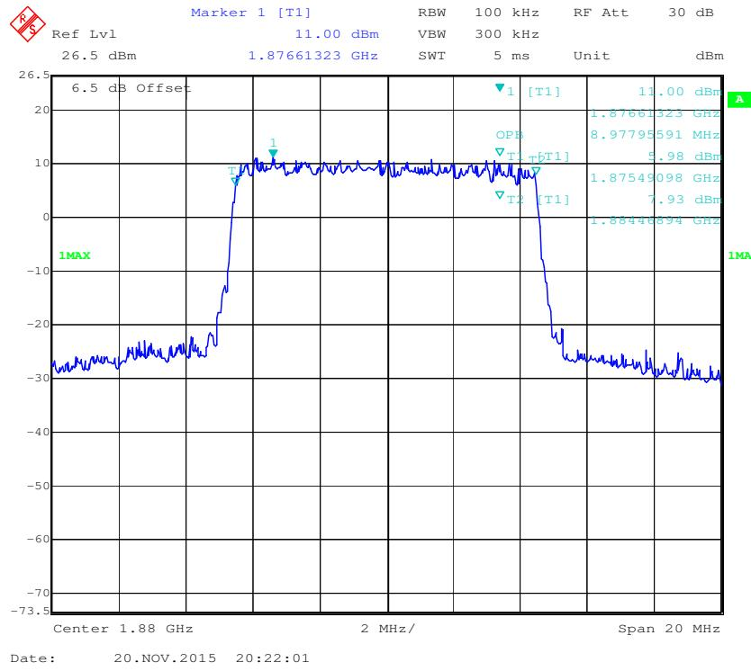
**16-QAM (10.0 MHz) - 99% Occupied Bandwidth, Middle channel**
