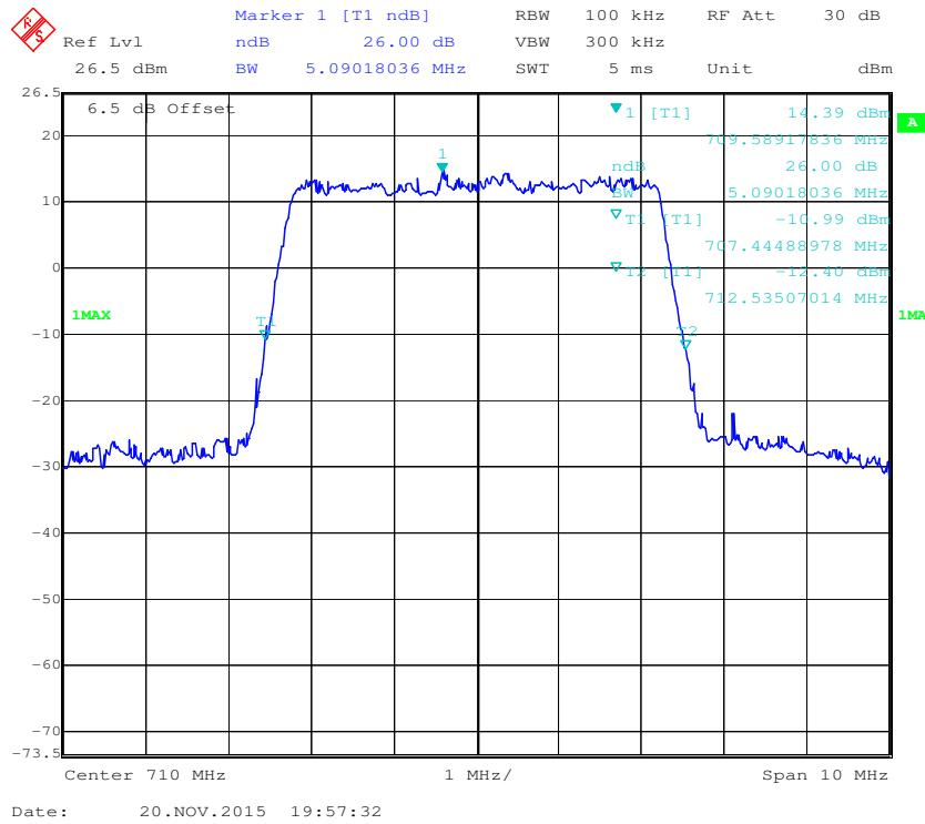
**QPSK (10.0 MHz) - 26 dB Bandwidth, Middle channel**
