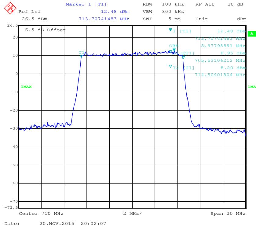
**QPSK (5.0 MHz) - 26 dB Bandwidth, Middle channel**
