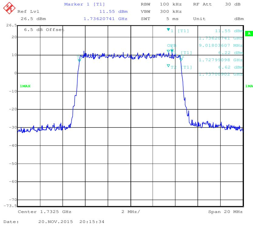
**16-QAM (10.0 MHz) - 99% Occupied Bandwidth, Middle channel**
