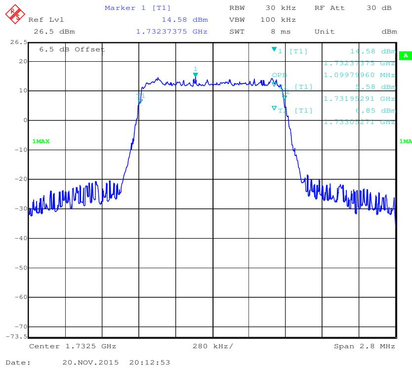
**16-QAM (1.4 MHz) - 99% Occupied Bandwidth, Middle channel**
