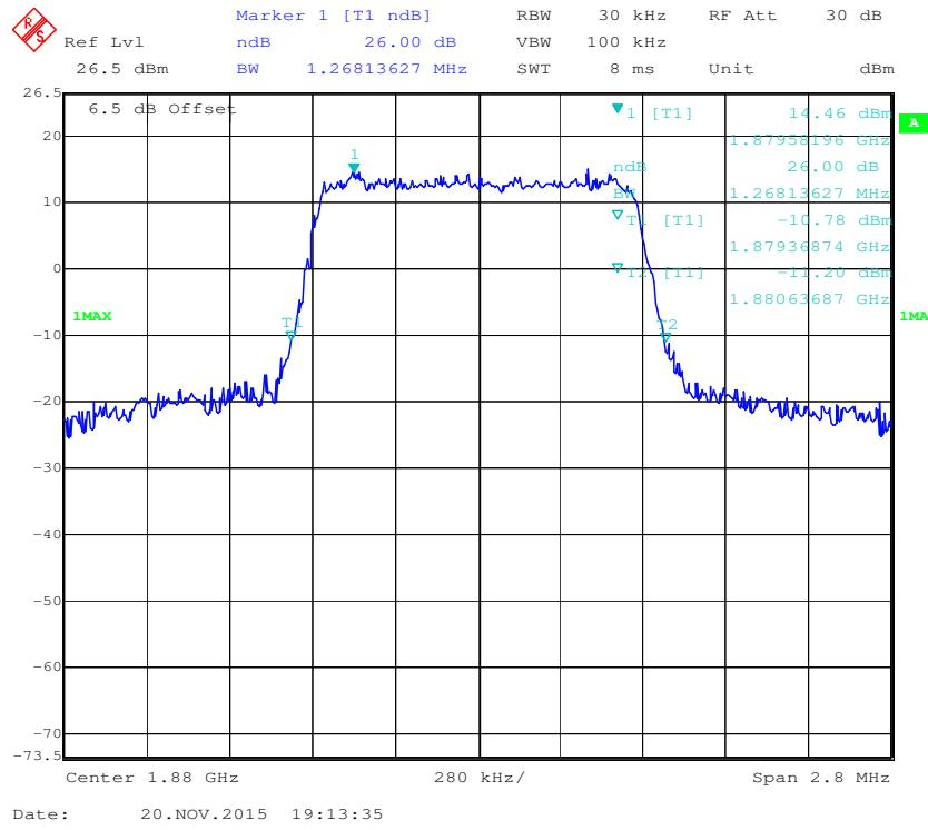
**16-QAM (1.4 MHz) - 26 dB Bandwidth, Middle channel**
