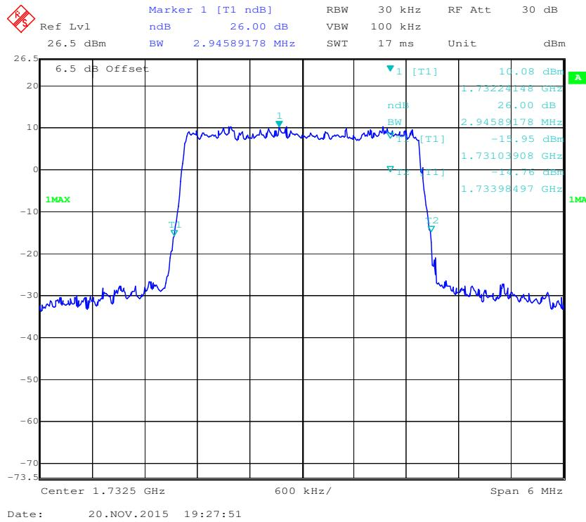
**QPSK (5.0 MHz) - 26 dB Bandwidth, Middle channel**
