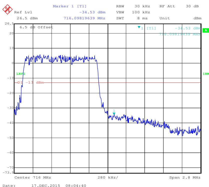
**16-QAM (1.4 MHz, FULL RB) - Left Band Edge**
