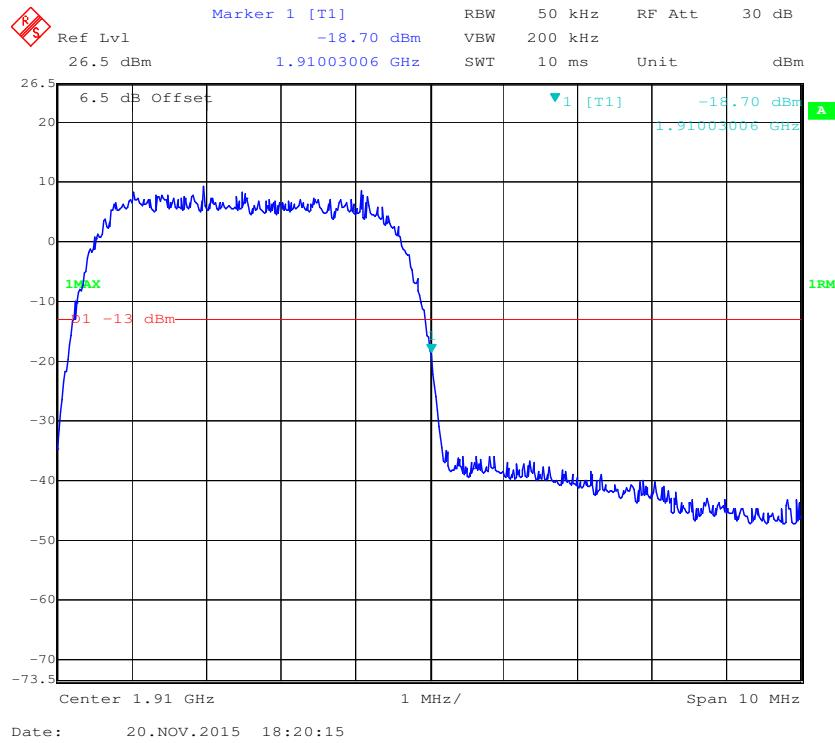
**PCS Band, Left Band Edge for HSUPA (BPSK) Mode**
