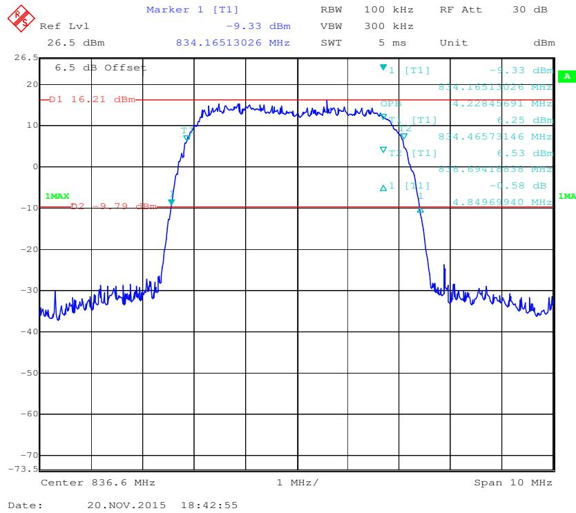
**99% Occupied &26 dB Emissions Bandwidth for HSDPA (16QAM) Mode**
