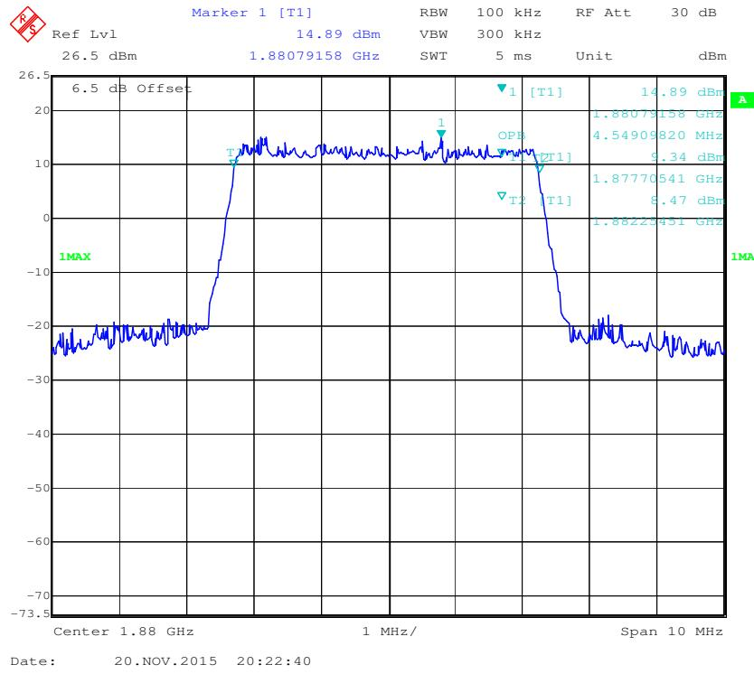
**16-QAM (5.0 MHz) - 99% Occupied Bandwidth, Middle channel**
