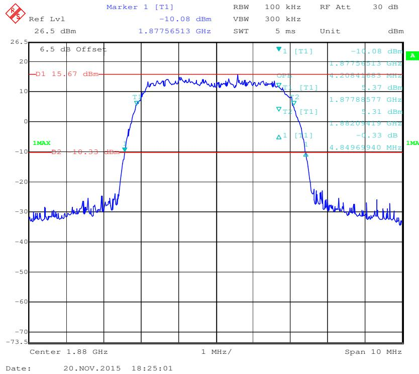
**AWS Band (Part 27)****99% Occupied & 26 dB Emissions Bandwidth for WCDMA (BPSK) Mode**
