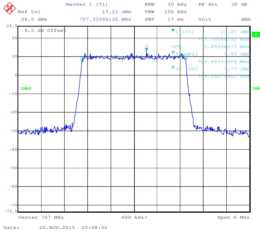
**16-QAM (3.0 MHz) - 99% Occupied Bandwidth, Middle channel**
