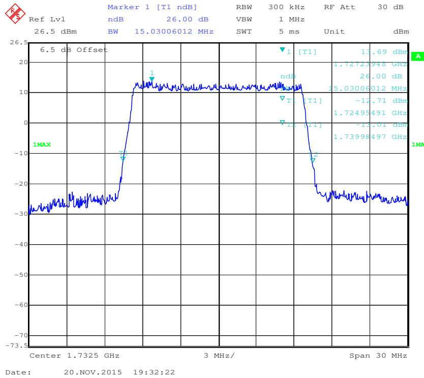
**QPSK (20.0 MHz) - 26 dB Bandwidth, Middle channel**
