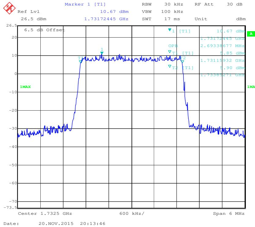
**QPSK (5.0 MHz) - 99% Occupied Bandwidth, Middle channel**
