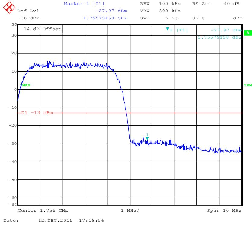
**AWS Band, Left Band Edge for HSDPA (16QAM) Mode**
