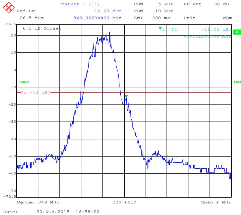
**Cellular Band, Left Band Edge for EGPRS Mode**
