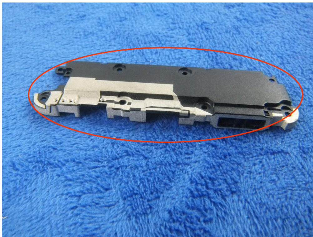
GSM/PCS/UMTS-FDD Antenna View
