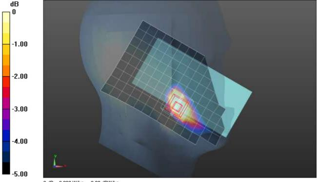
Frequency: 3646.7 MHz; Duty Cycle: 1:1.59956; Room Ambient Temperature: 24.0°C; Liquid Temperature: 23.0°C Medium parameters used (interpolated): f = 3646.7 MHz;  $\sigma = 2.931$  S/m;  $\epsilon_r = 37.52$ ;  $\rho = 1000$  kg/m³ Dasy Configuration:
