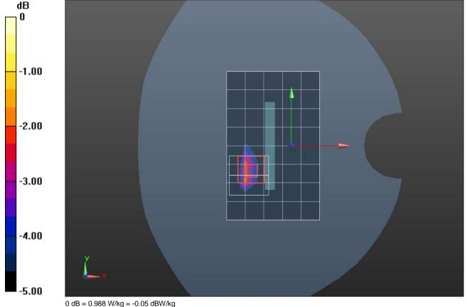
Frequency: 836.6 MHz; Duty Cycle: 1:1; Room Ambient Temperature: 24.0°C; Liquid Temperature: 23.0°C Medium parameters used (interpolated): f = 836.6 MHz;  $\sigma = 0.928$  S/m;  $\epsilon_r = 39.584$ ;  $\rho = 1000$  kg/m³ Dasy Configuration:
