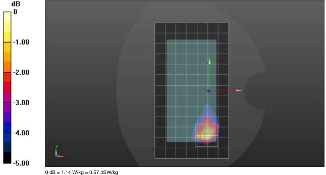
Frequency: 1882.5 MHz; Duty Cycle: 1:1; Room Ambient Temperature: 24.0°C; Liquid Temperature: 23.0°C Medium parameters used (interpolated): f = 1882.5 MHz;  $\sigma = 1.405$  S/m;  $\epsilon_r = 38.691$ ;  $\rho = 1000$  kg/m³ Dasy Configuration:
