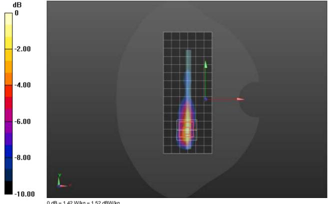
Frequency: 2489.3 MHz; Duty Cycle: 1:1; Room Ambient Temperature: 24.0°C; Liquid Temperature: 23.0°C Medium parameters used: f = 2490 MHz;  $\sigma$  = 1.808 S/m;  $\epsilon_r$  = 38.273;  $\rho$  = 1000 kg/m³ Dasy Configuration:
