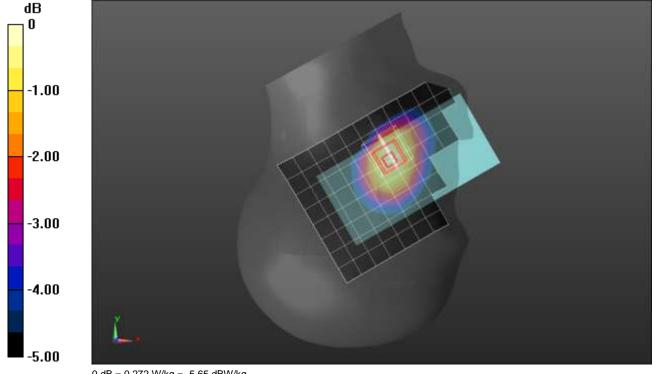
Frequency: 782 MHz; Duty Cycle: 1:1; Room Ambient Temperature: 24.0°C; Liquid Temperature: 23.0°C Medium parameters used (interpolated): f = 782 MHz;  $\sigma = 0.878$  S/m;  $\epsilon_r = 41.954$ ;  $\rho = 1000$  kg/m³ Dasy Configuration:
