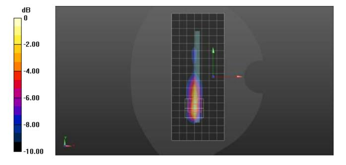
Frequency: 2441 MHz; Duty Cycle: 1:1; Room Ambient Temperature: 24.0°C; Liquid Temperature: 23.0°C Medium parameters used (interpolated): f = 2441 MHz;  $\sigma = 1.746$  S/m;  $\epsilon_r = 38.372$ ;  $\rho = 1000$  kg/m³ Dasy Configuration:
