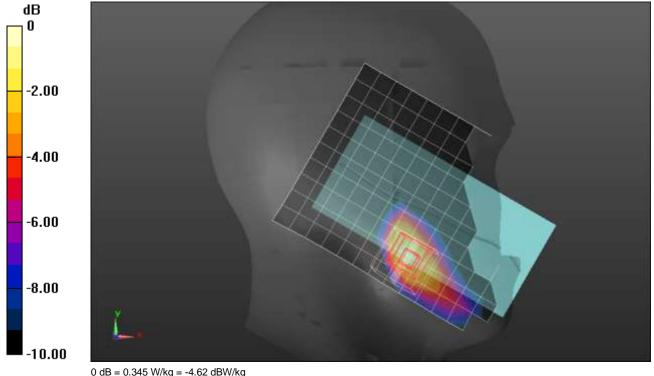
Frequency: 3499.98 MHz; Duty Cycle: 1:1; Room Ambient Temperature: 24.0°C; Liquid Temperature: 23.0°C Medium parameters used: f = 3500 MHz;  $\sigma = 2.783$  S/m;  $\epsilon_r = 38.419$ ;  $\rho = 1000$  kg/m<sup>3</sup> Dasy Configuration:
