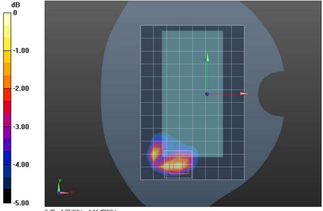
Frequency: 831.5 MHz; Duty Cycle: 1:1; Room Ambient Temperature: 24.0°C; Liquid Temperature: 23.0°C Medium parameters used (interpolated): f = 831.5 MHz;  $\sigma = 0.926$  S/m;  $\epsilon_r = 39.596$ ;  $\rho = 1000$  kg/m³ Dasy Configuration:
