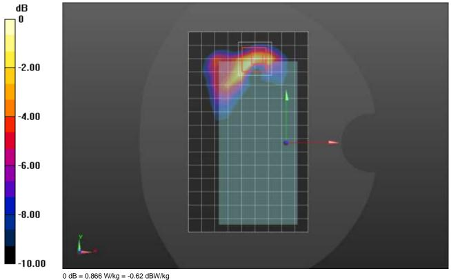
Frequency: 2593 MHz; Duty Cycle: 1:1; Room Ambient Temperature: 24.0°C; Liquid Temperature: 23.0°C Medium parameters used (interpolated): f = 2593 MHz;  $\sigma = 1.891 \text{ S/m}$ ;  $\epsilon_r = 37.23$ ;  $\rho = 1000 \text{ kg/m}^3$ Dasy Configuration:
