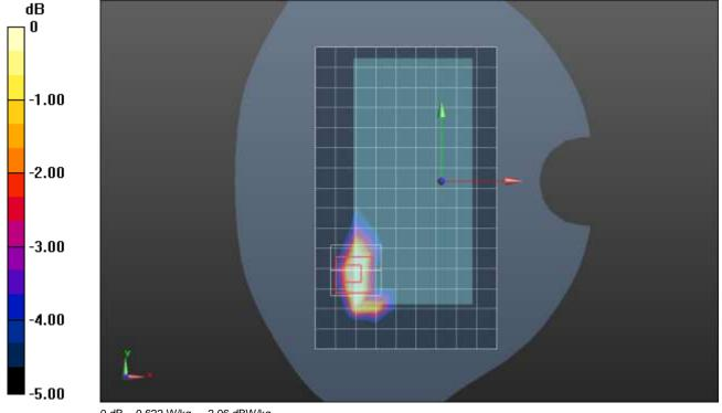
Frequency: 3690 MHz; Duty Cycle: 1:1.59956; Room Ambient Temperature: 24.0°C; Liquid Temperature: 23.0°C Medium parameters used: f = 3690 MHz;  $\sigma$  = 2.991 S/m;  $\varepsilon_r$  = 36.751;  $\rho$  = 1000 kg/m<sup>3</sup> Dasy Configuration:
