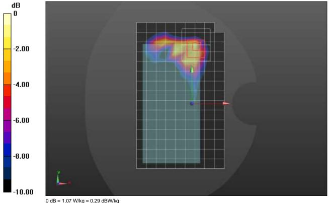
Frequency: 2535 MHz; Duty Cycle: 1:1; Room Ambient Temperature: 24.0°C; Liquid Temperature: 23.0°C Medium parameters used: f = 2535 MHz;  $\sigma = 1.85$  S/m;  $\varepsilon_r = 37.334$ ;  $\rho = 1000$  kg/m<sup>3</sup> Dasy Configuration:
