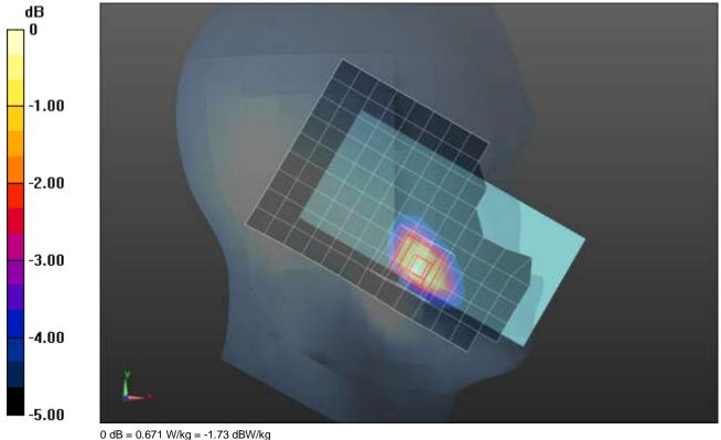
Frequency: 2535 MHz; Duty Cycle: 1:1; Room Ambient Temperature: 24.0°C; Liquid Temperature: 23.0°C Medium parameters used: f = 2535 MHz;  $\sigma$  = 1.924 S/m;  $\epsilon_r$  = 37.286;  $\rho$  = 1000 kg/m³ Dasy Configuration:
