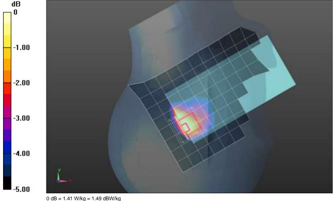
Frequency: 707.5 MHz; Duty Cycle: 1:1; Room Ambient Temperature: 24.0°C; Liquid Temperature: 23.0°C Medium parameters used (interpolated): f = 707.5 MHz;  $\sigma = 0.895$  S/m;  $\epsilon_r = 42.646$ ;  $\rho = 1000$  kg/m³ Dasy Configuration:
