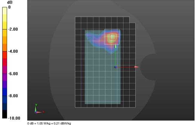
Frequency: 3840 MHz; Duty Cycle: 1:1; Room Ambient Temperature: 24.0°C; Liquid Temperature: 23.0°C Medium parameters used: f = 3840 MHz;  $\sigma$  = 3.119 S/m;  $\varepsilon_r$  = 36.958;  $\rho$  = 1000 kg/m<sup>3</sup> Dasy Configuration:
