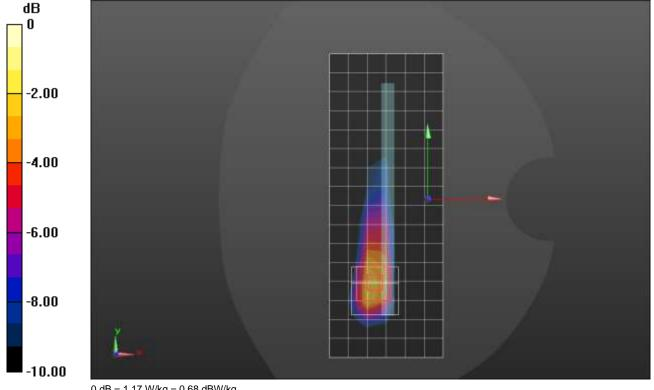
Frequency: 3840 MHz; Duty Cycle: 1:1; Room Ambient Temperature: 24.0°C; Liquid Temperature: 23.0°C Medium parameters used: f = 3840 MHz;  $\sigma = 3.101$  S/m;  $\varepsilon_r = 38.512$ ;  $\rho = 1000$  kg/m<sup>3</sup> Dasy Configuration:
