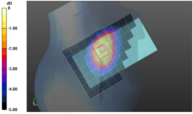
Frequency: 836.6 MHz; Duty Cycle: 1:1; Room Ambient Temperature: 24.0°C; Liquid Temperature: 23.0°C Medium parameters used (interpolated): f = 836.6 MHz;  $\sigma = 0.913$  S/m;  $\epsilon_r = 40.072$ ;  $\rho = 1000$  kg/m³ Dasy Configuration:
