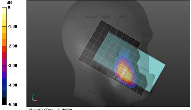
Frequency: 1745 MHz; Duty Cycle: 1:1; Room Ambient Temperature: 24.0°C; Liquid Temperature: 23.0°C Medium parameters used: f = 1745 MHz;  $\sigma$  = 1.405 S/m;  $\epsilon_r$  = 38.953;  $\rho$  = 1000 kg/m³ Dasy Configuration:
