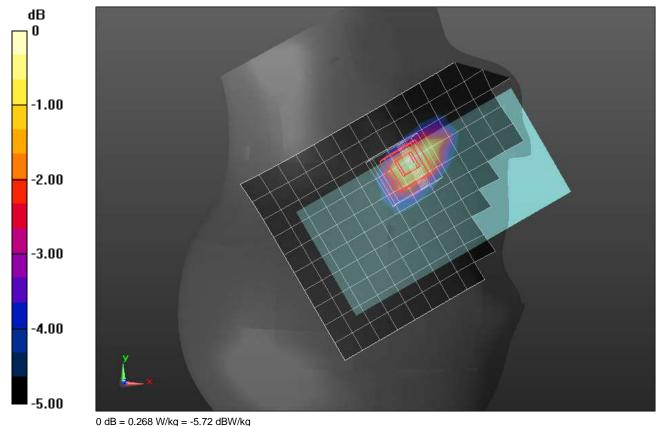
Frequency: 2489.3 MHz; Duty Cycle: 1:1; Room Ambient Temperature: 24.0°C; Liquid Temperature: 23.0°C Medium parameters used: f = 2490 MHz;  $\sigma = 1.808 \text{ S/m}$ ;  $\varepsilon_r = 38.273$ ;  $\rho = 1000 \text{ kg/m}^3$ Dasy Configuration:
