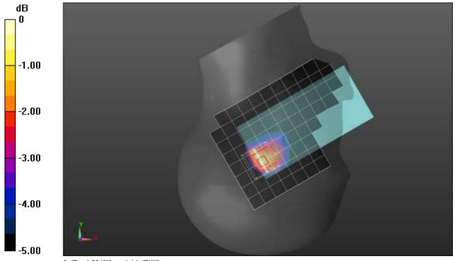
Frequency: 831.5 MHz; Duty Cycle: 1:1; Room Ambient Temperature: 24.0°C; Liquid Temperature: 23.0°C Medium parameters used (interpolated): f = 831.5 MHz;  $\sigma = 0.926$  S/m;  $\epsilon_r = 39.596$ ;  $\rho = 1000$  kg/m³ Dasy Configuration:
