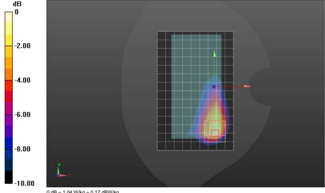
Frequency: 2560 MHz; Duty Cycle: 1:1; Room Ambient Temperature: 24.0°C; Liquid Temperature: 23.0°C Medium parameters used: f = 2560 MHz;  $\sigma = 1.983$  S/m;  $\varepsilon_r = 37.908$ ;  $\rho = 1000$  kg/m<sup>3</sup> Dasy Configuration:
