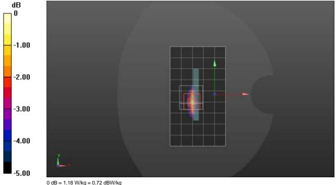
Frequency: 1745 MHz; Duty Cycle: 1:1; Room Ambient Temperature: 24.0°C; Liquid Temperature: 23.0°C Medium parameters used: f = 1745 MHz;  $\sigma = 1.388$  S/m;  $\varepsilon_r = 41.353$ ;  $\rho = 1000$  kg/m<sup>3</sup> Dasy Configuration:
