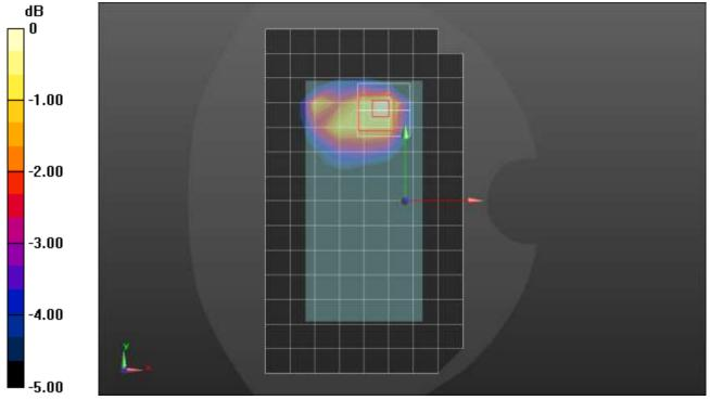
Frequency: 2310 MHz; Duty Cycle: 1:1; Room Ambient Temperature: 24.0°C; Liquid Temperature: 23.0°C Medium parameters used: f = 2310 MHz;  $\sigma$  = 1.696 S/m;  $\epsilon_r$  = 41.252;  $\rho$  = 1000 kg/m³ Dasy Configuration:
