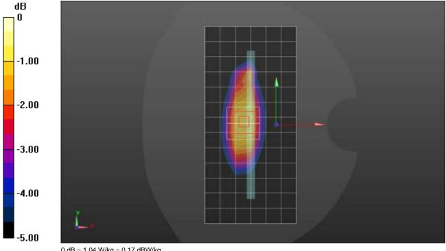
Frequency: 782 MHz; Duty Cycle: 1:1; Room Ambient Temperature: 24.0°C; Liquid Temperature: 23.0°C Medium parameters used (interpolated): f = 782 MHz;  $\sigma = 0.891$  S/m;  $\epsilon_r = 42.741$ ;  $\rho = 1000$  kg/m³ Dasy Configuration:
