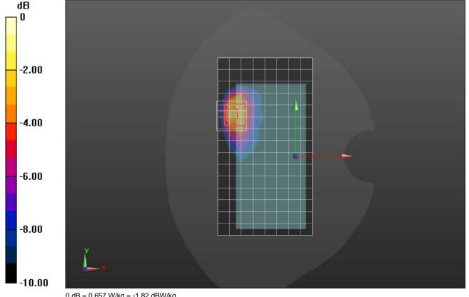
Frequency: 3499.98 MHz; Duty Cycle: 1:1; Room Ambient Temperature: 24.0°C; Liquid Temperature: 23.0°C Medium parameters used: f = 3500 MHz;  $\sigma = 2.86$  S/m;  $\epsilon_r = 37.445$ ;  $\rho = 1000$  kg/m³ Dasy Configuration:
