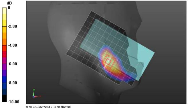
Frequency: 3840 MHz; Duty Cycle: 1:1; Room Ambient Temperature: 24.0°C; Liquid Temperature: 23.0°C Medium parameters used: f = 3840 MHz;  $\sigma$  = 3.104 S/m;  $\varepsilon_r$  = 39.399;  $\rho$  = 1000 kg/m<sup>3</sup> Dasy Configuration:
