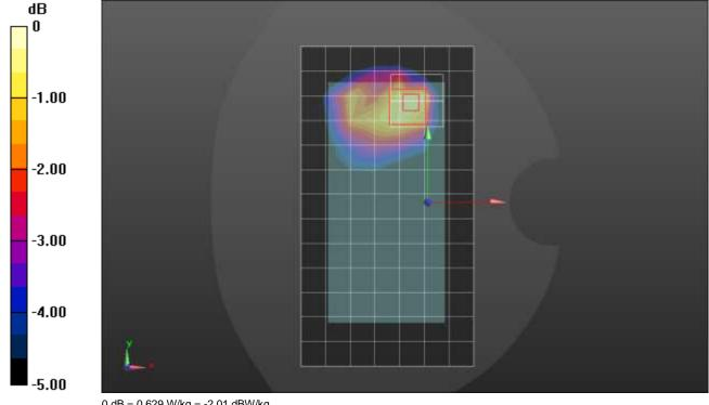
Frequency: 793 MHz; Duty Cycle: 1:1; Room Ambient Temperature: 24.0°C; Liquid Temperature: 23.0°C Medium parameters used (interpolated): f = 793 MHz;  $\sigma = 0.882$  S/m;  $\epsilon_r = 41.915$ ;  $\rho = 1000$  kg/m³ Dasy Configuration:
