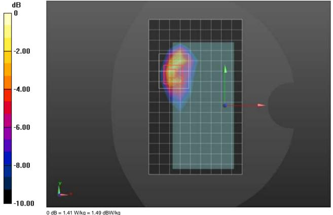
Frequency: 2535 MHz; Duty Cycle: 1:1; Room Ambient Temperature: 24.0°C; Liquid Temperature: 23.0°C Medium parameters used: f = 2535 MHz;  $\sigma = 1.877$  S/m;  $\epsilon_r = 37.735$ ;  $\rho = 1000$  kg/m³ Dasy Configuration:
