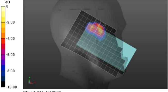
Frequency: 2593 MHz; Duty Cycle: 1:1.59956; Room Ambient Temperature: 24.0°C; Liquid Temperature: 23.0°C Medium parameters used (interpolated): f = 2593 MHz;  $\sigma$  = 1.994 S/m;  $\epsilon_r$  = 40.602;  $\rho$  = 1000 kg/m³ Dasy Configuration:
