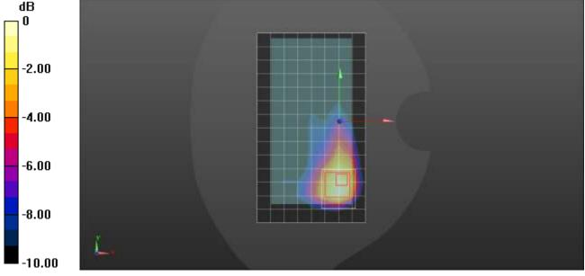
Frequency: 2441 MHz; Duty Cycle: 1:1; Room Ambient Temperature: 24.0°C; Liquid Temperature: 23.0°C Medium parameters used (interpolated): f = 2441 MHz;  $\sigma = 1.811$  S/m;  $\epsilon_r = 39.962$ ;  $\rho = 1000$  kg/m³ Dasy Configuration:
