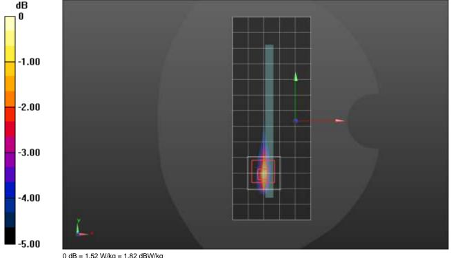
Frequency: 680.5 MHz; Duty Cycle: 1:1; Room Ambient Temperature: 24.0°C; Liquid Temperature: 23.0°C Medium parameters used (interpolated): f = 680.5 MHz;  $\sigma = 0.895$  S/m;  $\epsilon_r = 40.421$ ;  $\rho = 1000$  kg/m³ Dasy Configuration:
