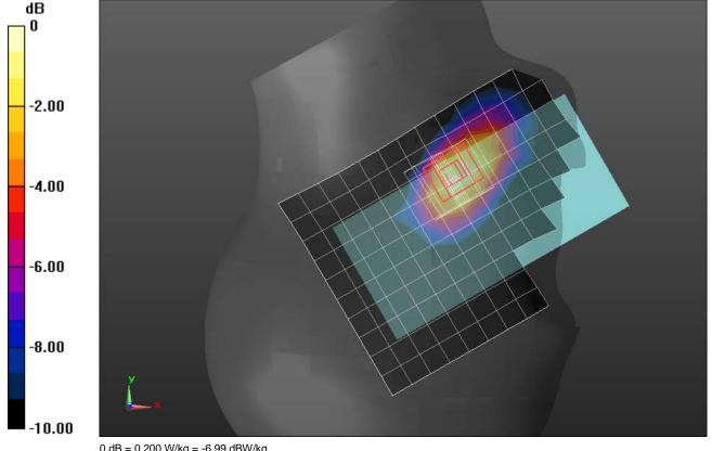
Frequency: 2489.2 MHz; Duty Cycle: 1:1.59956; Room Ambient Temperature: 24.0°C; Liquid Temperature: 23.0°C Medium parameters used: f = 2490 MHz;  $\sigma$  = 1.795 S/m;  $\epsilon_r$  = 37.829;  $\rho$  = 1000 kg/m³ Dasy Configuration:
