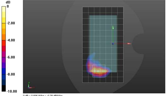
Frequency: 1720 MHz; Duty Cycle: 1:1; Room Ambient Temperature: 24.0°C; Liquid Temperature: 23.0°C Medium parameters used: f = 1720 MHz;  $\sigma$  = 1.389 S/m;  $\epsilon_r$  = 39.004;  $\rho$  = 1000 kg/m³ Dasy Configuration:
