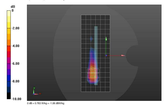
Frequency: 1617.6 MHz; Duty Cycle: 1:2.60976; Room Ambient Temperature: 24.0°C; Liquid Temperature: 23.0°C Medium parameters used (interpolated): f = 1617.6 MHz;  $\sigma = 1.275$  S/m;  $\epsilon_r = 38.644$ ;  $\rho = 1000$  kg/m³ Dasy Configuration:
