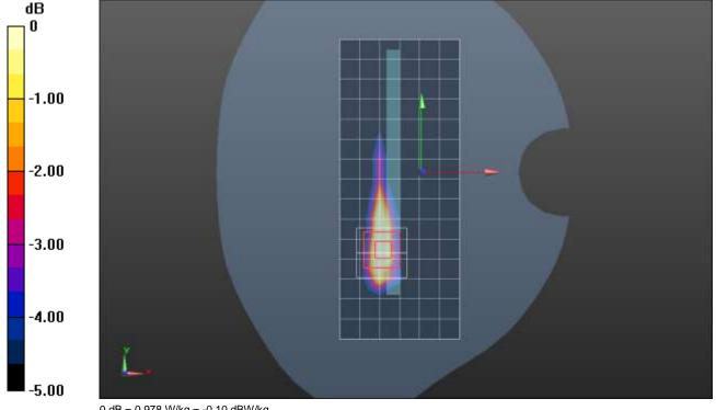
Frequency: 3690 MHz; Duty Cycle: 1:1.59956; Room Ambient Temperature: 24.0°C; Liquid Temperature: 23.0°C Medium parameters used: f = 3690 MHz;  $\sigma = 2.954$  S/m;  $\epsilon_r = 38.888$ ;  $\rho = 1000$  kg/m³ Dasy Configuration:
